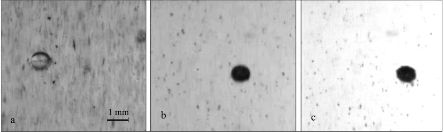
9. Images of toner ink adsorption to a single suspended bubble in a sodium oleate solution at a pH of 9.5 (a) immediately after ink injection, (b) 5 min after injection, and (c) 25 min after injection.
