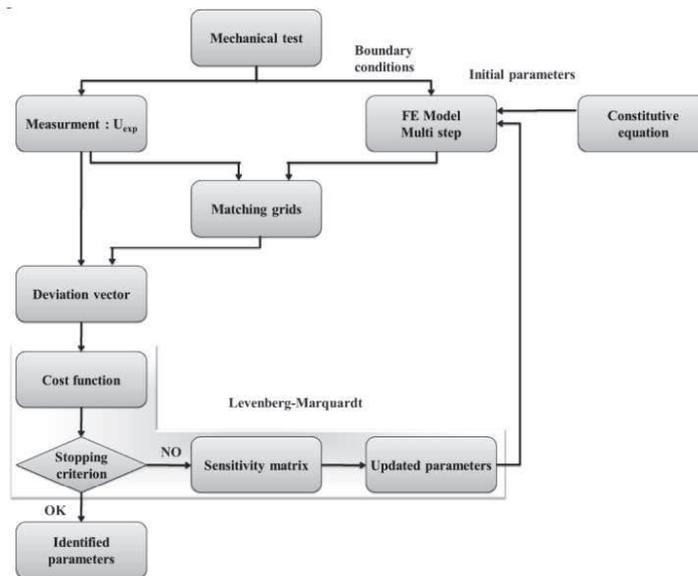
Figure 1: Identification procedure based on FEMU technique [3].
