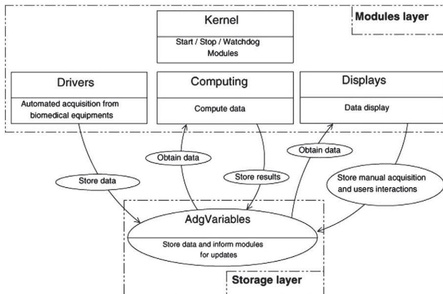
Fig. 4. Architecture of the *Aiddiag*'s software [4].
