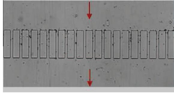
Fig. 3.  $\phi = 10^{-3} \text{ v/v}$ ;  $q = 2 \text{ ml h}^{-1}$ : no deposit of particles after 90 min of dead-end filtration. Latex suspensions are dispersed in ultra-pure water.
