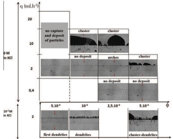
**Fig. 12.** Summary of different deposit structures of latex particles formed during filtration experiments. For  $q \leq 2$  ml h<sup>-1</sup>, images are taken after 90 min of filtration while experiments performed at  $q = 10$  ml h<sup>-1</sup> last only 40 min.
