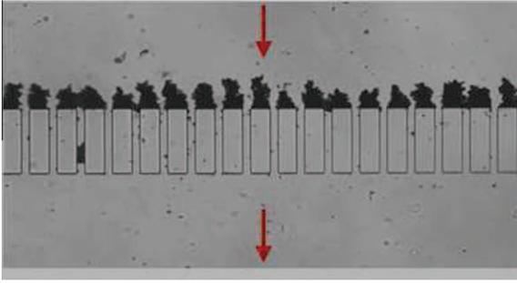
**Fig. 9.**  $\phi = 10^{-3}$  v/v;  $q = 2$  ml h<sup>-1</sup>: formation of straight dendrites after 90 min of dead-end filtration. Latex particles are dispersed in KCl-water solution at  $10^{-1}$  M.
