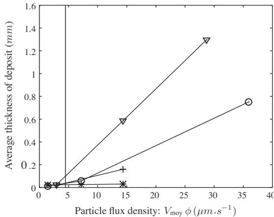
**Fig. 14.** Determination of a critical flux density of particle leading to the deposition and to the microsystem clogging after 90 min of dead-end filtration. Each symbol corresponds to a different volume fraction of latex particles dispersed in ultra-pure water, \* :  $\phi = 5.10^{-4}$ ,  $\diamond$  :  $\phi = 10^{-3}$ ,  $\circ$  :  $\phi = 2.510^{-3}$ , and + :  $\phi = 5.10^{-3}$ .
