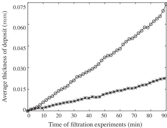
**Fig. 11.** The temporal evolution of the average thickness of particle deposit: --  $\phi = 10^{-3}$  v/v;  $q = 2$  ml h<sup>-1</sup> (dispersed in ultra-pure water), and --  $\phi = 10^{-3}$  v/v;  $q = 2$  ml h<sup>-1</sup> (dispersed in KCl at  $10^{-1}$  M).
