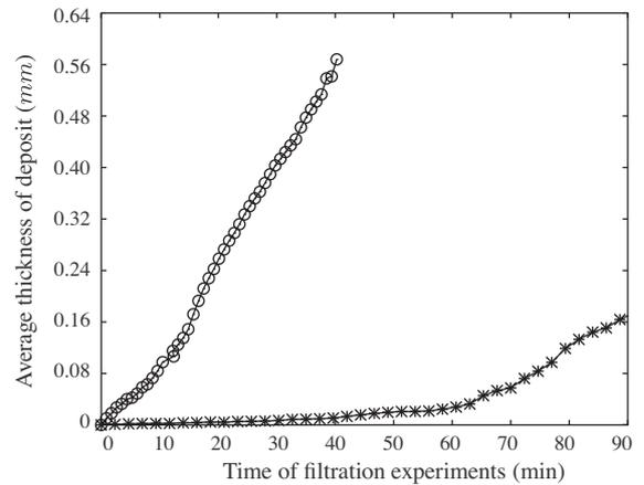
**Fig. 7.** The temporal evolution of the average thickness of particle deposit:  $-\ast-$   $\phi = 5.10^{-3}$  v/v;  $q = 2$  ml  $h^{-1}$ , and  $-o-$   $\phi = 10^{-3}$  v/v;  $q = 10$  ml  $h^{-1}$  (dispersed in ultra-pure water).
