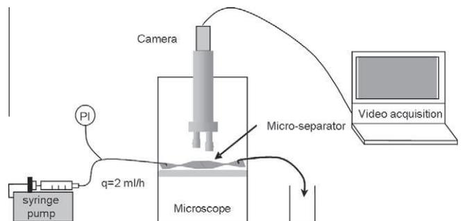
Fig. 2. Experimental set-up for imaging the channel blockage.
