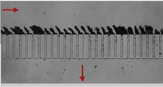
**Fig. 10.**  $\phi = 10^{-3}$  v/v;  $q = 2$  ml h<sup>-1</sup>: formation of tilted dendrites after 90 min of cross-flow filtration. Latex particles are dispersed in KCl-water solution at  $10^{-1}$  M.
