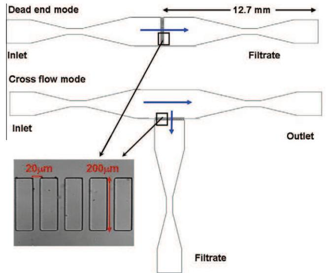
Fig. 1. Schematic view of the PDMS micro-separators used for dead-end and cross-flow filtration.
