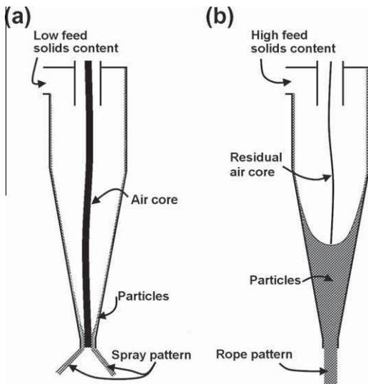
Fig. 1. Hydrocyclone: (a) dilute and (b) dense slurries.
