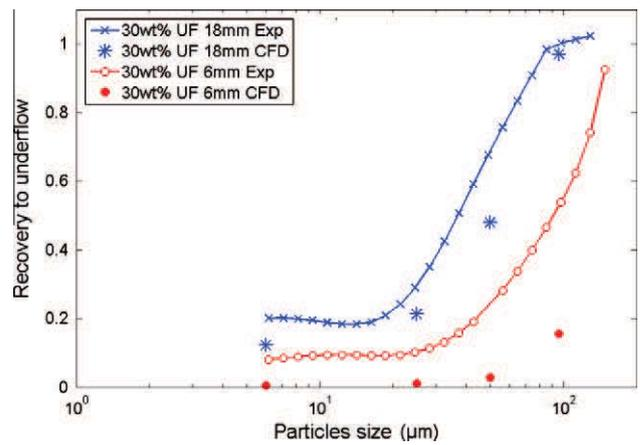
Fig. 15. Influence of spigot diameter on separation curves.
