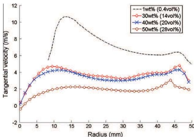
**Fig. 10.** Water tangential velocity profile in the cylindrical section of the hydrocyclone, taken 100 mm under the roof.
