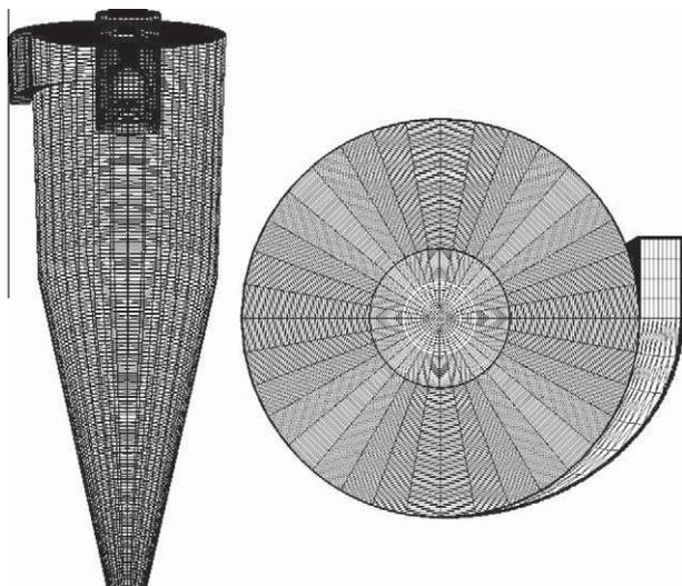
Fig. 2. Axial and cross-section view of the mesh.
