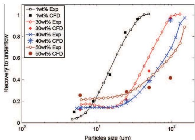
Fig. 9. CFD predictions of separation curve as a function of feed solids concentration (symbols: simulation, solid lines: experimental measurements).
