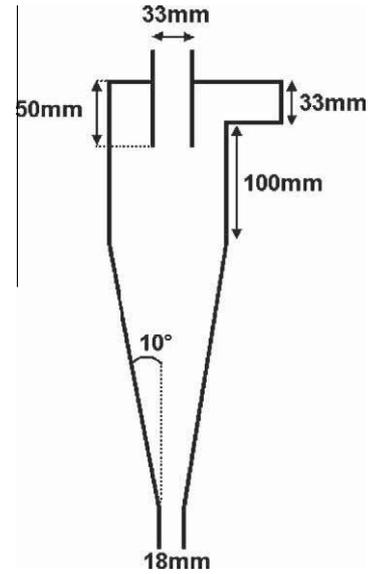
Fig. 3. Geometric features of Neyrtec's HC100 hydrocyclone.
