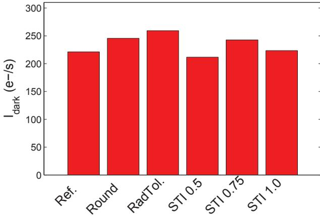
Fig. 13. Dark current of the alternative photodiode layouts after 75 krad(SiO<sub>2</sub>) with  $V_{LOTG} = -0.6$  V. The differences between structures are small enough to be attributed to device mismatches and measurement errors.
