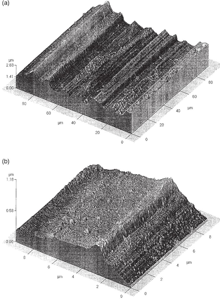
Fig. 3. AFM images of 512×512 points of the alloy sheet surface. (a) at 100 μm<sup>2</sup> scale; (b) at 10 μm<sup>2</sup> scale.
