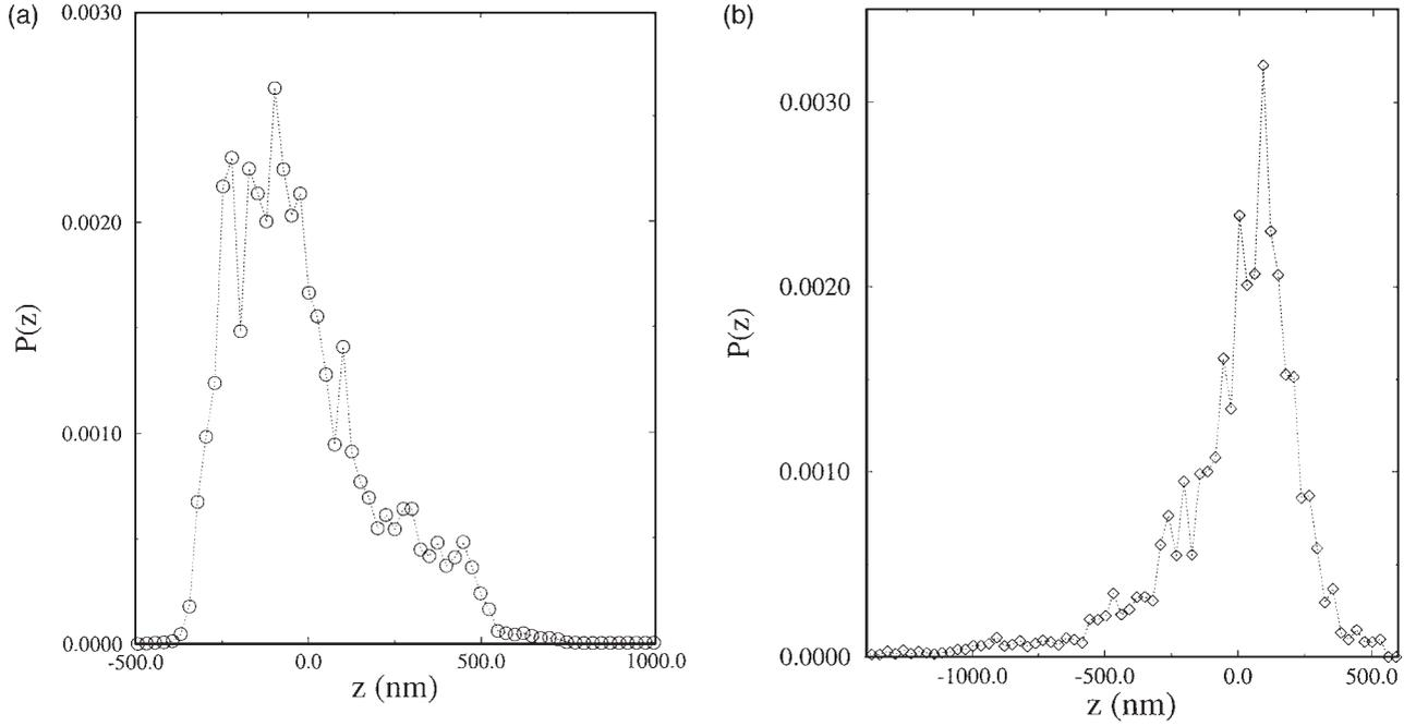
Fig. 5. Height distribution is computed from averaging five  $100 \mu\text{m}^2$  surfaces of  $512 \times 512$  points. (a)  $\circ$  for alloy sheet sample (2) being rolled-pass by the cylinder; (b)  $\diamond$  for steel roll.
