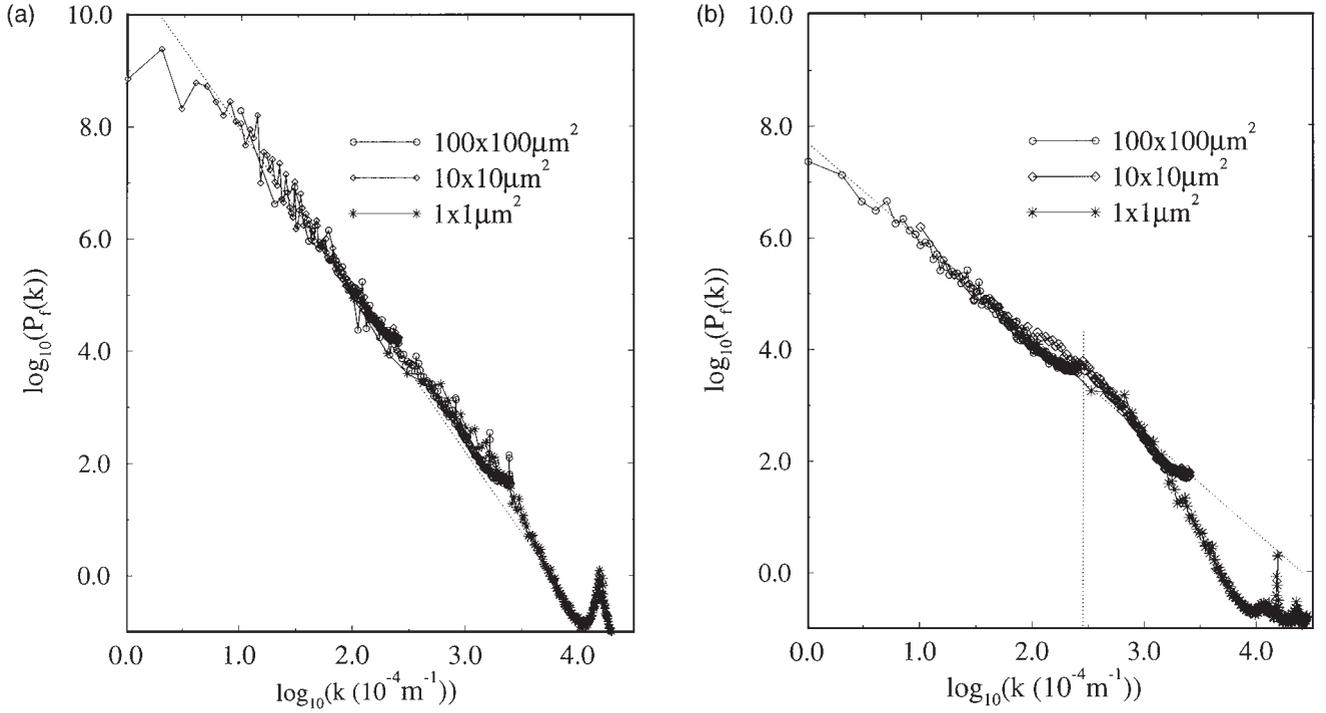
Fig. 6. Averaged power spectra of height profiles of the Al alloy sheet (No. 1) in log-log coordinates at different scales:  $\circ$   $10 \mu\text{m}$ ,  $\diamond$   $10 \mu\text{m}$ , and  $\star$   $1 \mu\text{m}$ . Dotted line indicates self-affine power law. (a) In transverse direction : the estimated transverse self-affine exponent is  $\zeta_{\perp} = 0.93 \pm 0.05$ ; (b) In longitudinal direction :  $\zeta_{\parallel} = 0.4 \pm 0.1$ .
