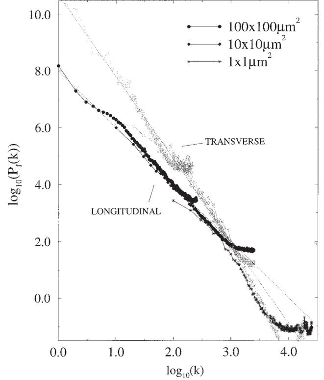
Fig. 8. Same conventions as Fig. 6 for the Al alloy sheet (No. 2). In transverse direction with grey points:  $\zeta_{\perp}=0.93\pm 0.05$  In longitudinal direction black points:  $\zeta_{\parallel}=0.5\pm 0.1$ .
