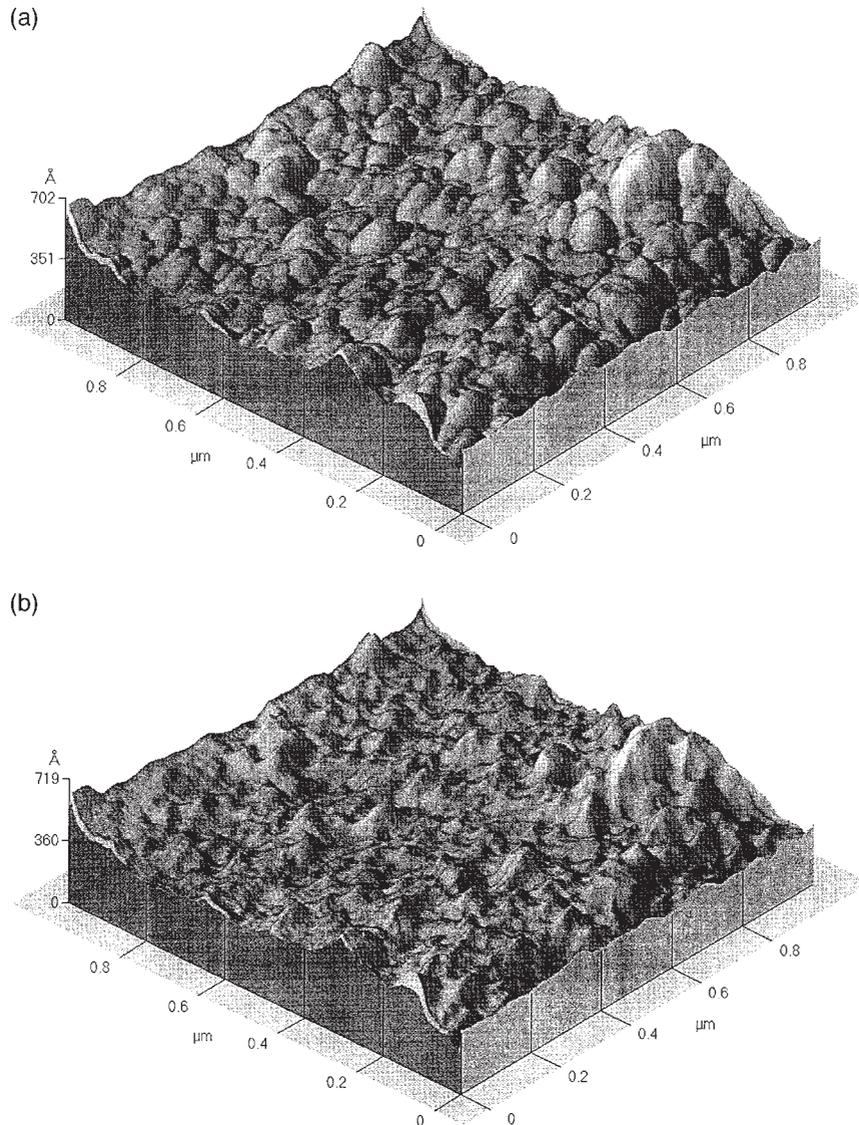
Fig. 2. AFM images of  $512 \times 512$  points of the alloy sheet surface at  $1 \mu\text{m}^2$  scale. (a) direct image from AFM measurements; (b) reconstructed image for a given 30 nm AFM tip diameter.
