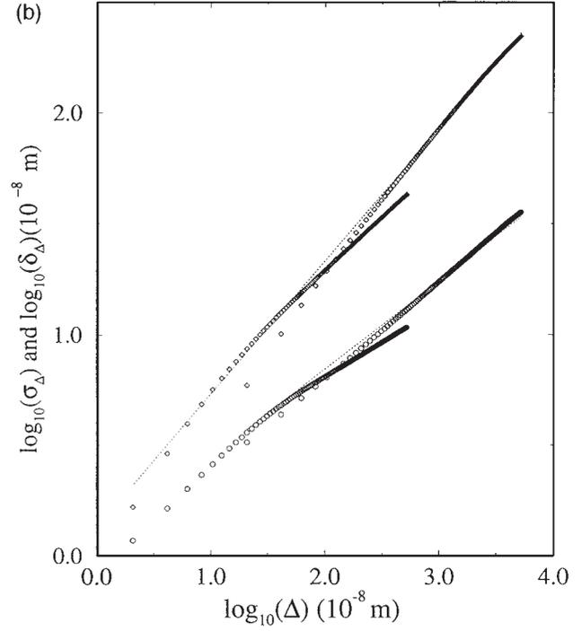
Fig. 10. Variable band width method is used to analyze the height profile of the alloy sheet sample (No. 1).  $\diamond$  Root mean square deviation  $\sigma$  and  $\circ$  min-max difference are plotted versus the window size  $\Delta$  in log-log coordinates (a) In transverse direction:  $\zeta_{\perp}=0.85\pm 0.07$ ; (b) In longitudinal direction:  $\zeta_{\parallel}=0.5\pm 0.1$ .
