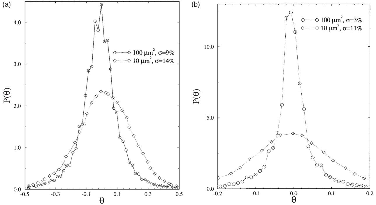
Fig. 14. Slope histogram for alloy sheets of type (No. 1) (a) in transverse direction  $\circ$  at  $l=100/512 \approx 0.2 \mu\text{m}$  scale,  $\diamond$  at  $l=10/512 \approx 0.02 \mu\text{m}$  scale; (b) in longitudinal direction, same conventions as (a).
