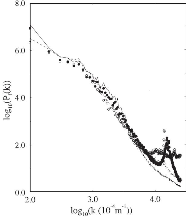
Fig. 7. Comparison of height power spectra between direct and eroded images of  $1\ \mu\text{m}^2$  size. Averaged power spectrum of 512 height profiles is shown in log-log coordinates for real data in transverse  $\bullet$  and longitudinal  $\circ$  directions, as well as for reconstructed profiles with full line in the transverse direction and dashed line in the longitudinal direction.
