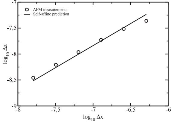
Fig. 3. Roughness analysis computed from AFM measurements (○) compared with predictions obtained via a fit of the angular scattered intensity distribution assuming self-affine correlations. The slope of the line is  $\zeta = 0.78$  and the amplitude parameter is  $s(\lambda) = 0.11$ .
