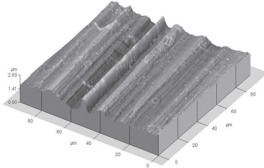
Fig. 1. AFM image of  $512 \times 512$  points of the aluminum alloy sheet surface. This image has been obtained by Plouraboué and Boehm [15] in contact mode on a Park Scientific AFM using a long range scanner ( $100 \mu\text{m}$  lateral travel and  $5 \mu\text{m}$  vertical travel). The height standard deviation has been measured to be  $\sigma = 2.5 \mu\text{m}$ .
