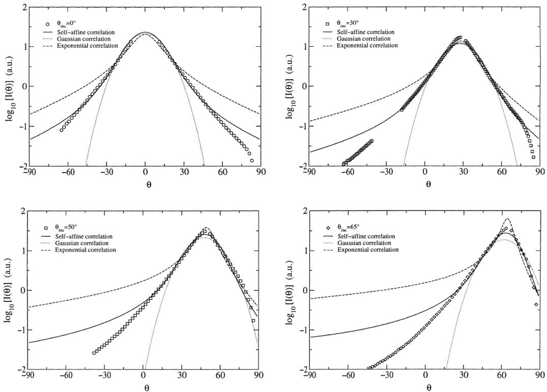
Fig. 2. Scattered intensity measurements obtained at incidence angles  $\theta_0 = 0^\circ$ ,  $30^\circ$ ,  $50^\circ$  and  $65^\circ$ , respectively. The experimental results are shown in symbols. The solid/dotted/dashed lines correspond to the expressions obtained for a Kirchhoff approximation in case of self-affine/Gaussian/exponential correlations, respectively.
