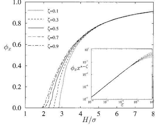
FIG. 10.  $\phi_x$  for a self-affine aperture. Hurst exponents ranging from 0.1 to 0.9 have been computed. The inset shows the numerical data collapse obtained using rescaling [Eq. (24)] near the contact.
