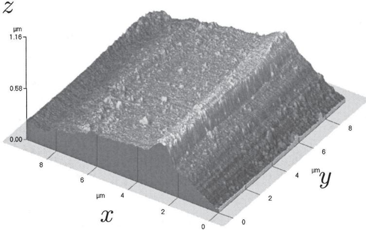
FIG. 1. An example of a microscopic view of an anisotropic surface topography from Ref. [12], using an atomic force microscope
