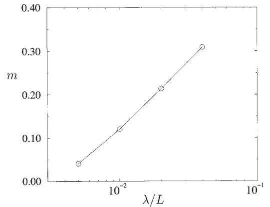
FIG. 9. Power-law coefficient  $m$  of the shear Couette flow factor vs the correlation length  $\lambda$  with the same convention as in Fig. 4. The dot size represents the error bars of the numerical computations.
