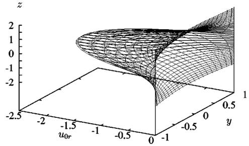
FIG. 3. The real part of the downstream velocity perturbation in the gas  $z > 0$  and in the liquid  $z < 0$  for  $Re=15$ . The nondimensionalizations of the gas and liquid velocities differ by the factor  $\mu_l/\mu_g$ .
