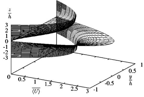
FIG. 1. The mean velocity in the gas  $z > 0$  and in the liquid  $z < 0$  normalized by their different gap-averaged values far from the interface,  $\langle U_g \rangle$  and  $\langle U_l \rangle$ , which differ by a factor  $\mu_l/\mu_g$ .
