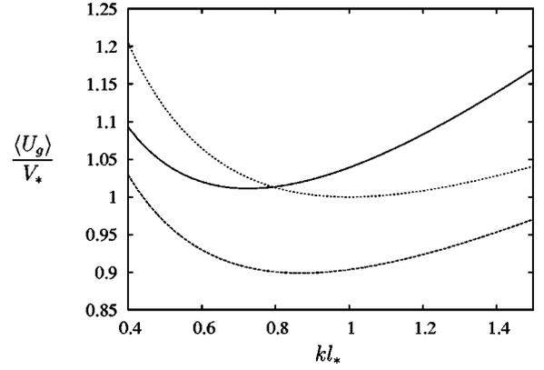
FIG. 9. The critical gas velocity  $U_g$  scaled by  $V_*$  as a function of the wavenumber  $k$  scaled by  $1/l_*$  for  $\text{Re}_* = 40$ . The continuous curve is the result for Eq. (18). The dashed curve is the corresponding result for our previous theory (Ref. 2) for the outer ignoring the existence of the inner meniscus region. The dotted curve is for the simple Euler–Darcy theory (Ref. 1).
