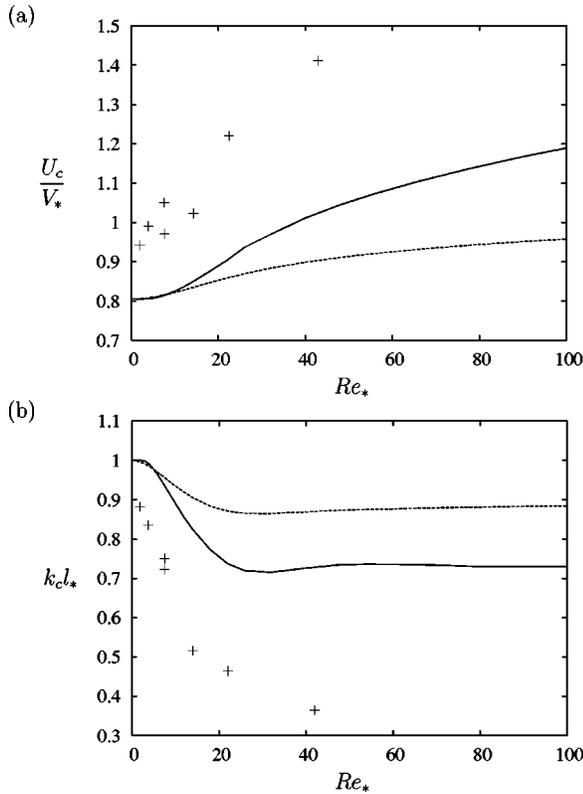
FIG. 10. (a) The minimum mean gas velocity  $U_c$  for an instability as a function of the Reynolds number  $Re_*$  and (b) the minimizing wavenumber  $k_c$ . The continuous curve is our new theory, while the dashed curve is the corresponding results of our previous theory. The points are experimental results (Ref. 3).
