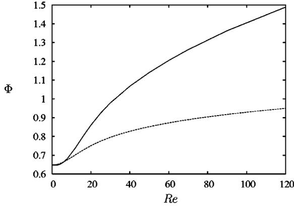
FIG. 8. The combination  $\Phi(\text{Re}) = \text{Re}/(-Q_{gr}P_r + Q_{gi}P_i - 3\Delta Q_{li})$  representing the reduction of the critical Kelvin–Helmholtz velocity. The broken curve is the corresponding result of our first paper (Ref. 2), in which we effectively took  $Q_g = 1$  and  $\Delta Q_l = 1$ .
