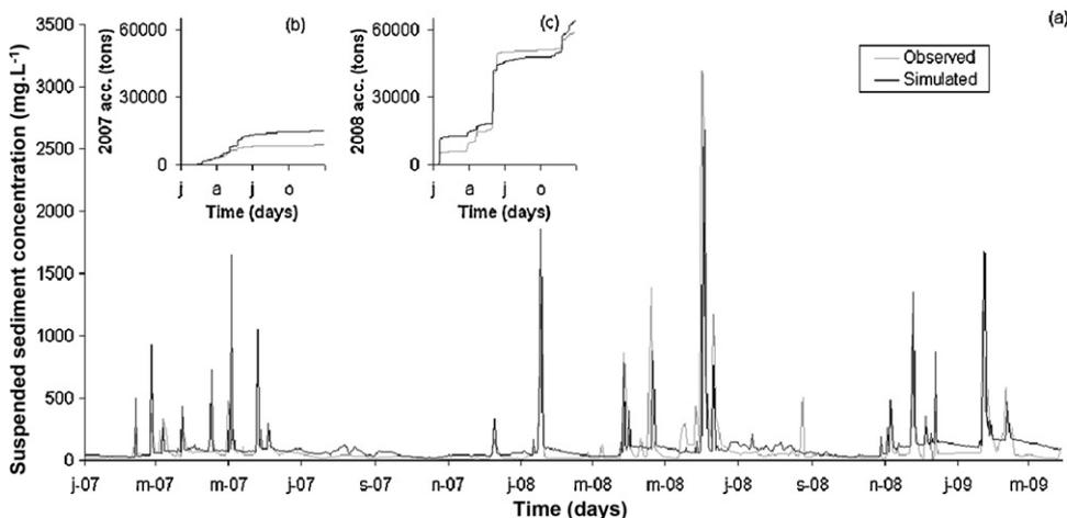
Fig. 4. Observed and simulated daily (a) suspended sediment concentration ( $\text{mg L}^{-1}$ ) at the Larra gauging station (January 2007–March 2009), (b) 2007 accumulation (tons) and (c) 2008 accumulation (tons).
