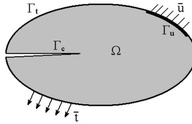
**Figure 1.** Notations for the 2D discontinuous body
