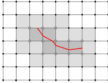
**Figure 4.** XFEM enriched mesh with a crack
