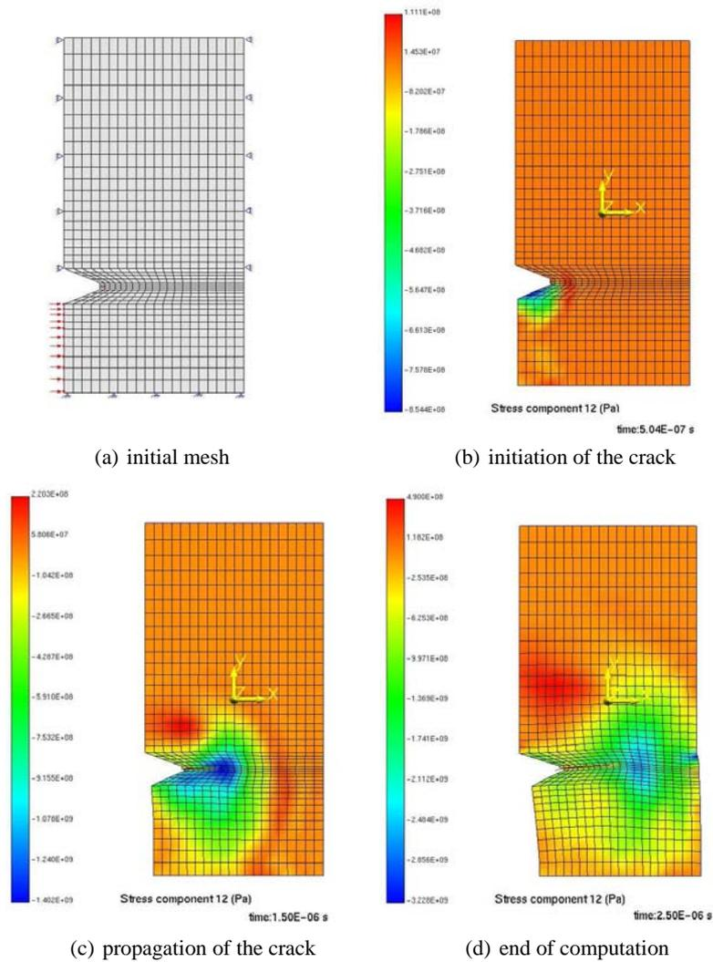
**Figure 7.** Numerical results for the fracture test model
