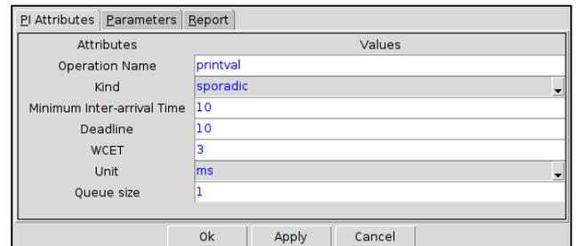
Figure 5- Timing Requirements of the sporadic interface *printval*
