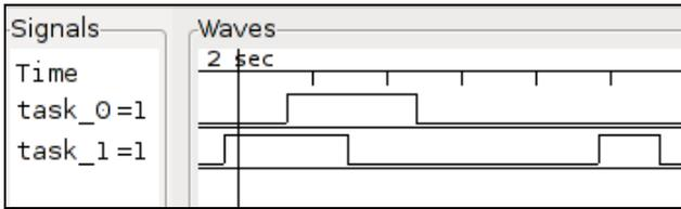
Figure 2- Graphical representation of VCD file using GTKWave
