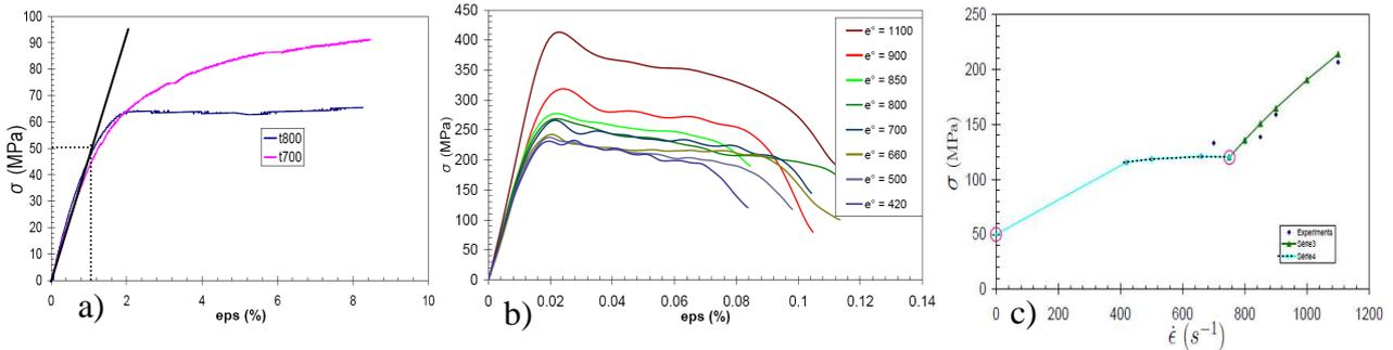
**Figure 1.** a) Quasi-static tension of T700/M21S and T800/M21S  $[\pm 45^\circ]_{2s}$ ; b) Dynamic compression of T800/M21S  $[\pm 45^\circ]_{3s}$ ; c) Strain rate effects on T800/M21S  $[\pm 45^\circ]_{2s}$  lamina strength.
