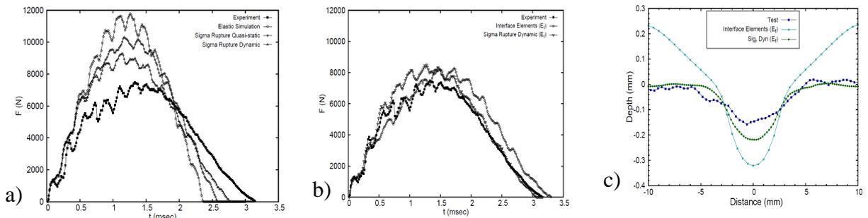
**Figures 2. a) and b) Force [N] versus time [ms] history curves; c) Indentations [mm].**
