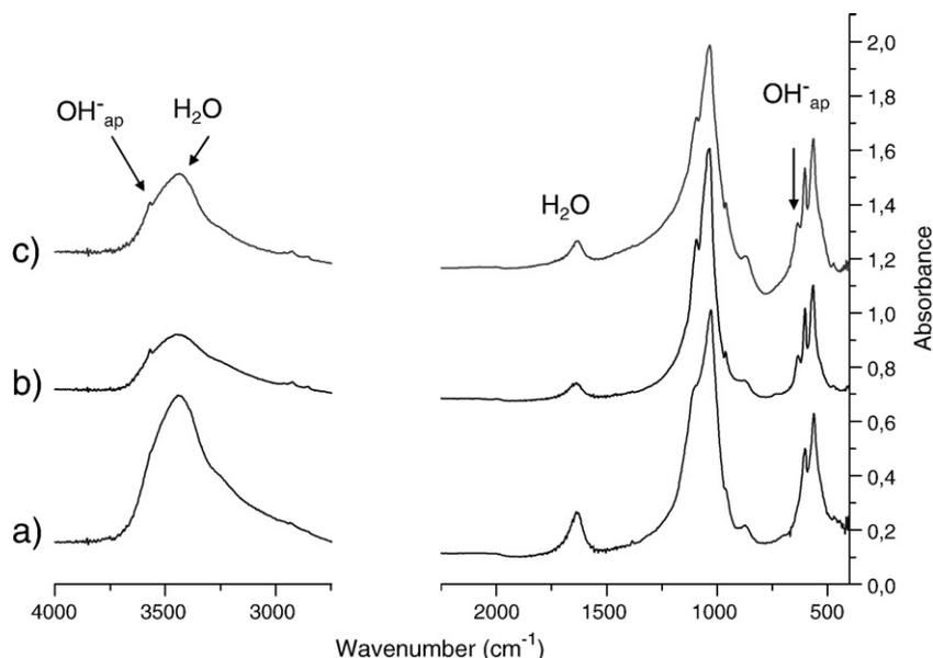
Fig. 6. FTIR spectra of a) initial powder, b) powder consolidated by uni-axial pressing at  $200^\circ\text{C}$  for 15 min and c) powder consolidated by SPS (under vacuum) at  $200^\circ\text{C}$  for 2 min.
