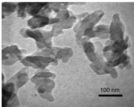
Fig. 5. TEM micrograph for typical nanocrystalline apatite morphology.
