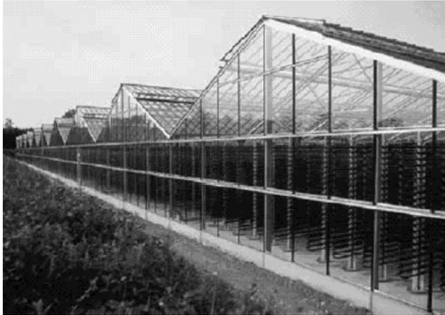
FIG. 4. Glass tube photobioreactor (700 m<sup>3</sup>) producing *Chlorella* biomass (Klötze, Germany).
