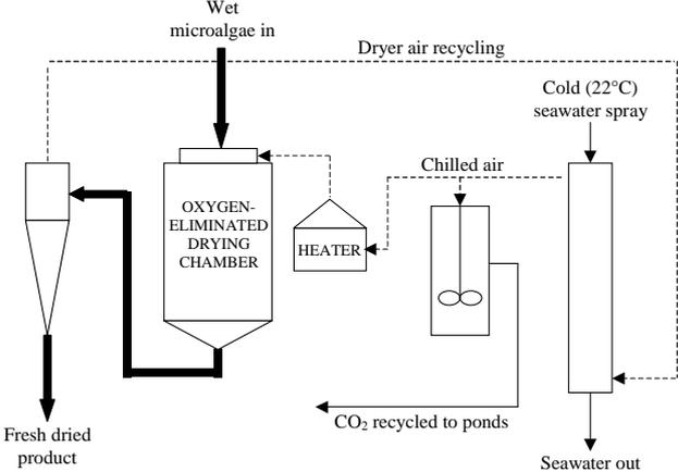
FIG. 3. Cyanotech process for drying microalgae biomass.
