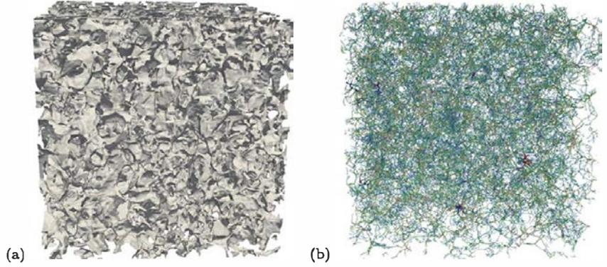
skeleton [16, 48] as implemented in CImg plugin [56] (see Fig. 1 for illustration). The skeleton will be used latter as the support for the EMA.
