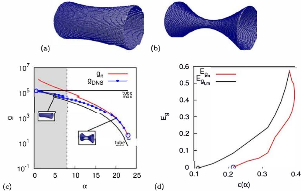
Fig. 7 Illustration of curvature corrected formula on an ideal throat. a and b exemplify two generated throats. a  $(R_o, \alpha) = (25, 5)$  and b  $(R_o, \alpha) = (25, 20)$ . c Variation of conductance values with respect to  $\alpha$  parameter either computed by curvature corrected formula (6) in red or (4) for maximal tube or minimal tube (resp. horizontal and decreasing black lines). d DNS relative error to a reference conductance versus
