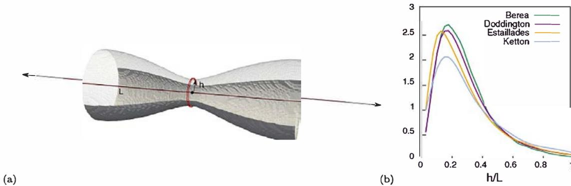
Fig. 2 a Illustration of the asymptotic requirement at the throat location for  $\epsilon = 0.04$ . b Distribution of the geometrical asymptotic constriction parameter  $\epsilon$  for the various samples ( $1000^3$  voxels images)
