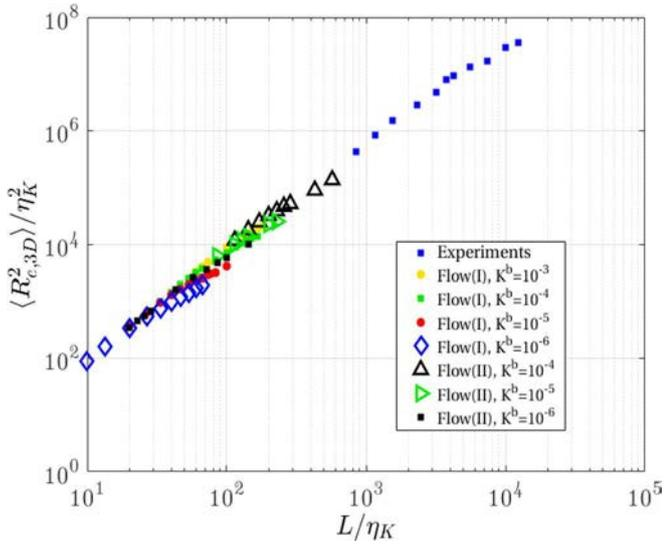
**Fig. 8.** Evolution of the end-to-end distance for fibers of different lengths  $L$ , bending rigidities  $K^b$  and flow parameters.  $\langle \mathbf{R}_{e,3D}^2 \rangle_t$  is scaled by the Kolmogorov length.
