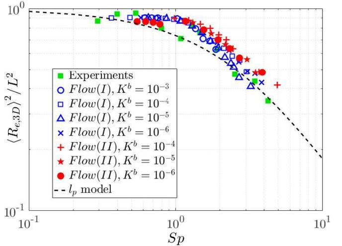
**Fig. 10.** Evolution of the dimensionless end-to-end distance with Sperm number. Comparison of  $\langle \mathbf{R}_{e,3D}^2 \rangle_t / L^2$  for simulations with  $\gamma = 3$ , experiments of [14] with  $\gamma = 2$ , and model of eq. (19) in dashed line.
