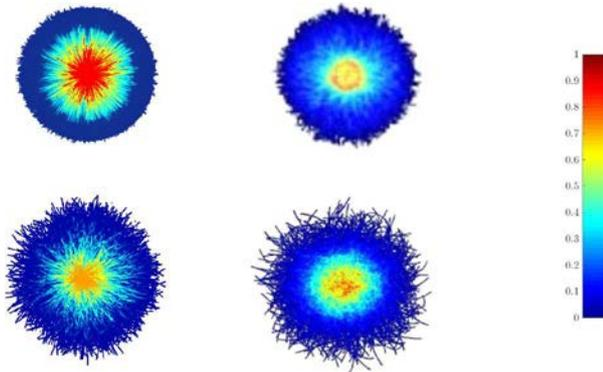
**Fig. 6.** Comparison between numerical simulations (left column) and experiments (right column) of fiber deformation for rigid regime (top row) and flexible regime (bottom row). Each fiber has one end positioned at the center of the graphic and color is proportional to the probability of finding one bead of the fiber at the considered position from the center.
