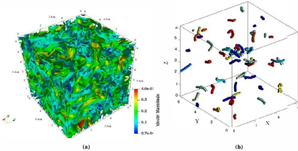
Fig. 5. (a) Visualization of Homogeneous Isotropic Turbulence for  $Re_\lambda = 51$  with velocity contours. (b) Snapshot of the fibers positions simulated in Homogeneous Isotropic Turbulence. The number of fibers is 45 with diameter  $d = 0.1$  and length  $L = 2$  discretized with 20 beads.
