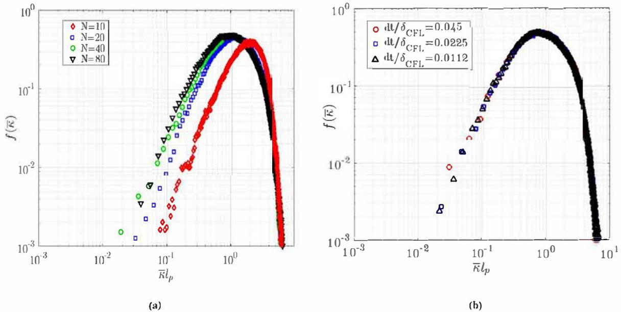
Fig. 2. Probability density functions of the mean curvature (eq. (11)) of fibers in turbulence. (a) Effect of fiber discretization into  $N$  beads on the determination of the curvature.  $l_p$  is the persistence length defined in eq. (15). (b) Effect of the time step on the numerical solution with  $N=20$ .  $\delta_{CFL}$  is the Courant-Friedrichs-Lewy reference time step.
