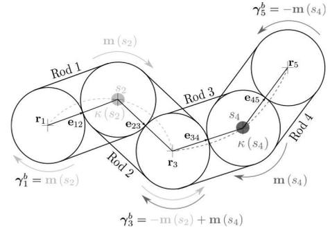
**Fig. 1.** Fiber discretization and bending torques acting on beads. The fiber is composed of spherical beads which stay in contact through no-slip rolling conditions. Two consecutive beads are forming a rod.
