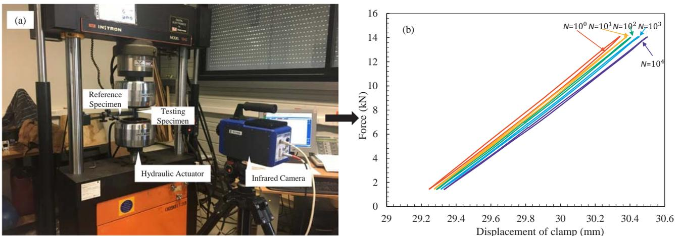
Fig. 5. (a) Experimental setup with infrared camera; (b) Typical hysteresis loops during fatigue tests of UD CRFP laminates.
