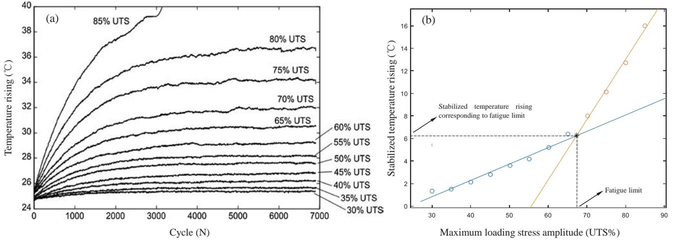
Fig. 6. Experimental data from [13]. (a) Temperature evolution curves; (b) Fatigue limit determination.
