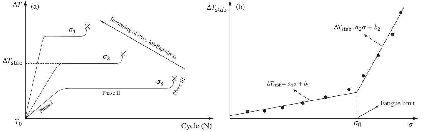
**Fig. 1.** Rapid determination of fatigue limit based on thermographic data. (a) Typical temperature evolution during fatigue test ( $T_0$ : initial temperature;  $\Delta T$ : temperature rising;  $\Delta T_{\text{stab}}$ : stabilized temperature rising;  $\sigma$ : maximum applied loading stress,  $\sigma_1 > \sigma_2 > \sigma_3$ ). (b) Fatigue limit determined by an improved method based on statistical analysis.
