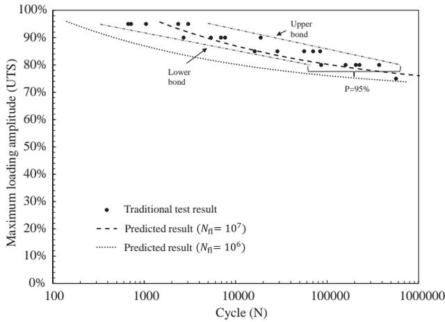
Fig. 12. Comparison of predicted S-N curves and traditional test results for UD CFRP laminates.
