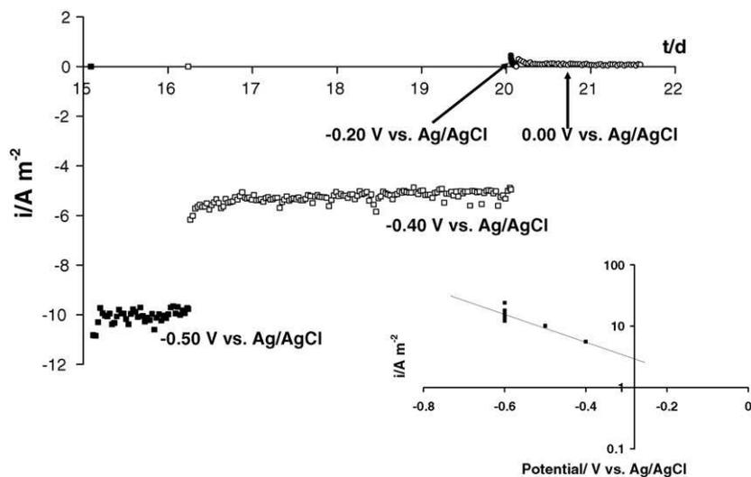
Fig. 4. Variation of the current density on electrode SS3.4 from reactor 3, previously kept in open circuit for 15 days and then consecutively polarized at ■  $-0.50 \text{ V}$  □  $-0.40 \text{ V}$  ●  $-0.20 \text{ V}$  ○  $0.00 \text{ V vs. Ag/AgCl}$ . Inset: current density obtained during the different electrolyses performed with stainless steel electrodes (values in Table 1) in logarithmic scale, as a function of potential.
