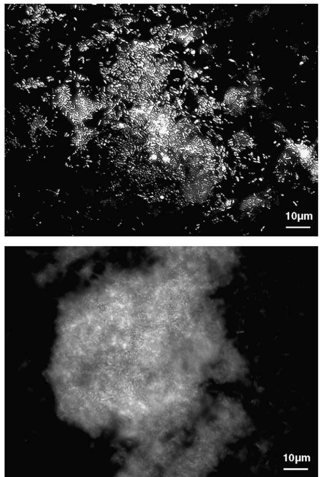
Fig. 3. Epifluorescence microscopy pictures of *G.sulfurreducens* biofilm on stainless steel electrode polarized at  $-0.60 \text{ V vs. Ag/AgCl}$  from reactor 2 (magnification  $500\times$ ), A: SS2.1; B: SS2.2.
