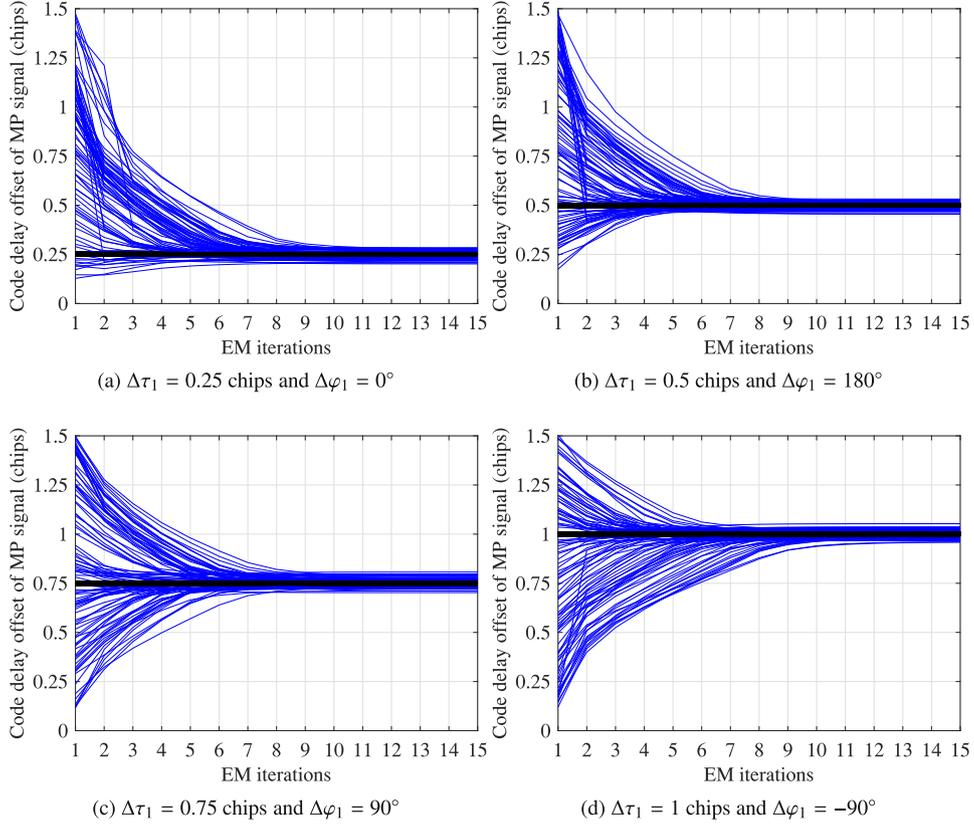
**Fig. 3.** Estimated MP code delay offset versus the number of EM iterations for 100 MC simulations. Estimated value: blue line; True value: black line. (For interpretation of the references to colour in this figure legend, the reader is referred to the web version of this article.)
