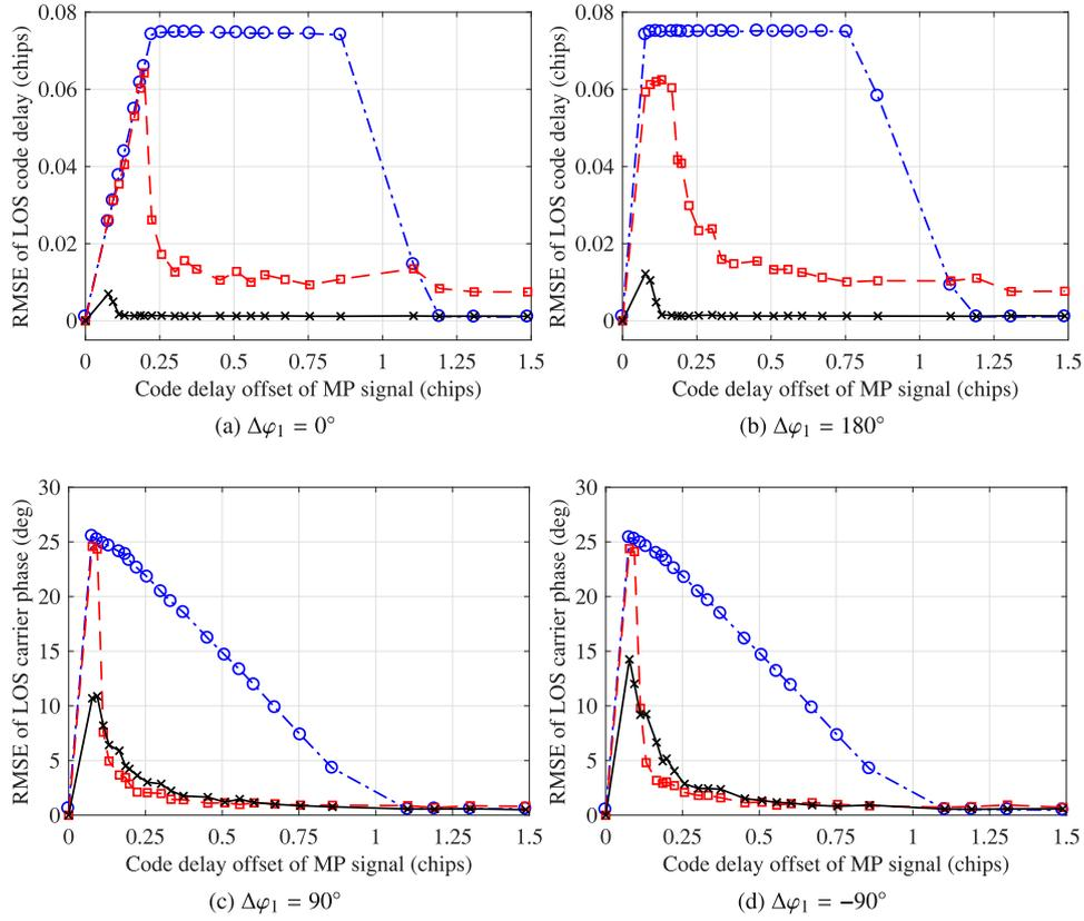
**Fig. 1.** RMSE envelopes of the LOS code delay and carrier phase with different approaches. Proposed approach: black solid line; FIMLA: red dashed line; Narrow correlator DLL: blue dash-dotted line. (For interpretation of the references to colour in this figure legend, the reader is referred to the web version of this article.)
