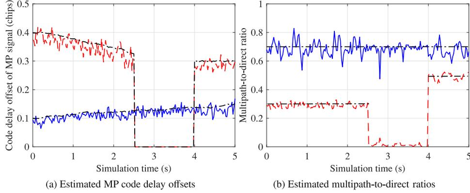
**Fig. 8.** Estimation results for two MP signal parameters in dynamic scenarios. MP #1: blue solid line; MP #2: red dashed line; True value: black dash-dotted line. (For interpretation of the references to colour in this figure legend, the reader is referred to the web version of this article.)
