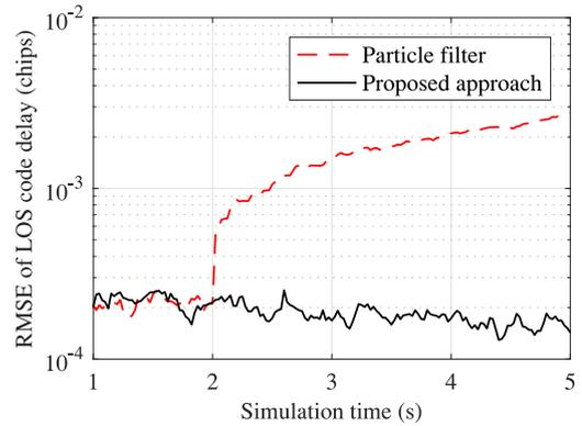
**Fig. 7.** RMSE of the estimated LOS code delay in the presence of changes affecting the dynamics of MP signals.**Table 4**
