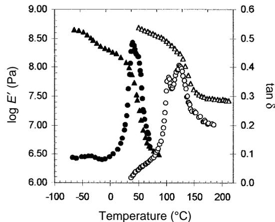
**FIG. 3.** DMTA data recorded at 5 Hz in bending mode. (▲), (●)  $\log E'$ ,  $\tan \delta$  for cellulose trioctanoate; (△), (○)  $\log E'$ ,  $\tan \delta$  for cellulose mixed acetic-octanoic triester ( $DS_{\text{acetyl}} = 2.19$ ;  $DS_{\text{octanoyl}} = 0.81$ ). See Figure 1 for abbreviation.
