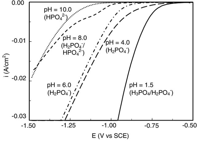
Fig. 3. Voltammery curves (scan rate = 20 mV/s) obtained with stainless steel rotating disk electrode (1000 rpm) in solutions at different pH with 150 mM phosphate and 100 mM KCl as supporting electrolyte. Predominant phosphate species are indicated for each curve.
