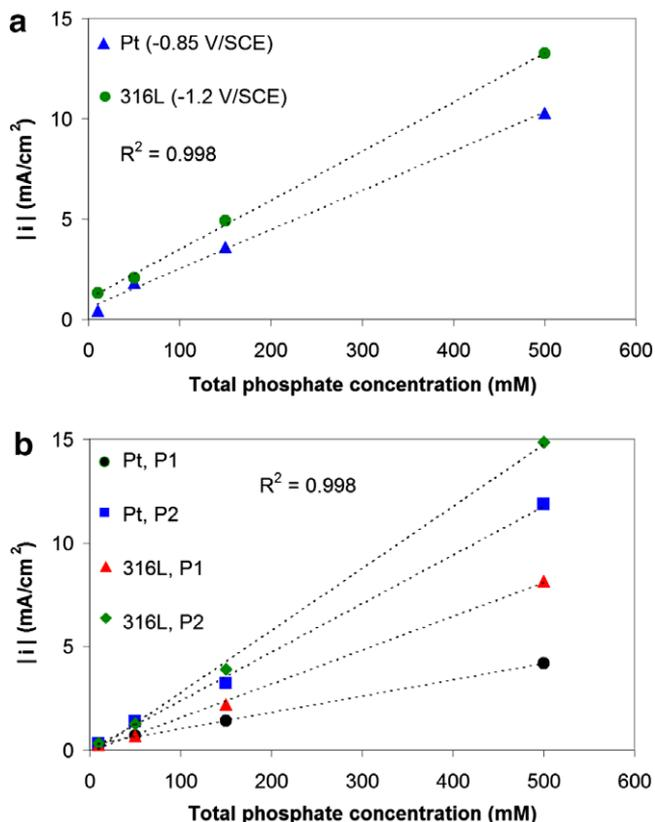
Fig. 2. (a) Current density vs. phosphate concentration at  $-0.85$  V/SCE for platinum from Fig. 1a and at  $-1.20$  V/SCE for 316L stainless steel from Fig. 1b. (b) Current density vs. phosphate concentration at the first (P1) and second (P2) inflection points of the waves from Fig. 1a and b for platinum and 316L stainless steel.
