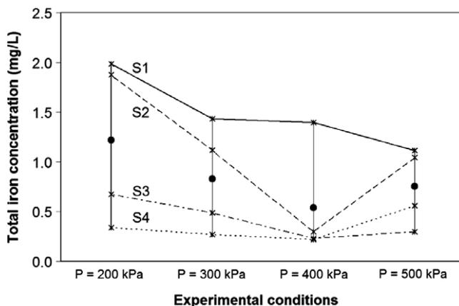
Fig. 7. Experimental (\*) and average (●) values of the total iron concentration released after a 3 h immersion of a mild steel coupon in a 1 mM phosphate solution with hydrogen gas under different pressures: 200, 300, 400 and 500 kPa (absolute) which correspond approximately to the dissolved hydrogen concentrations of 1.5, 2.3, 3.1, 3.8 mM respectively. Four identical series of experiments were performed (S1, S2, S3 and S4).
