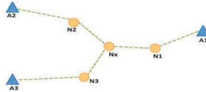
Fig. 1. Localization with the 3D DV-HOP + RSSI protocol
