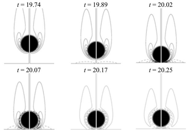
**Fig. 1.** Iso-vorticity contours from  $-17.8$  to  $17.8$  of a sphere bouncing on a wall with  $\rho_p/\rho = 8$ ,  $St = 53$  and  $Re \approx 60$ . Positive (resp. negative) values are continuous (resp. dashed) lines. Images are inspired from [11] and have been mirrored.
