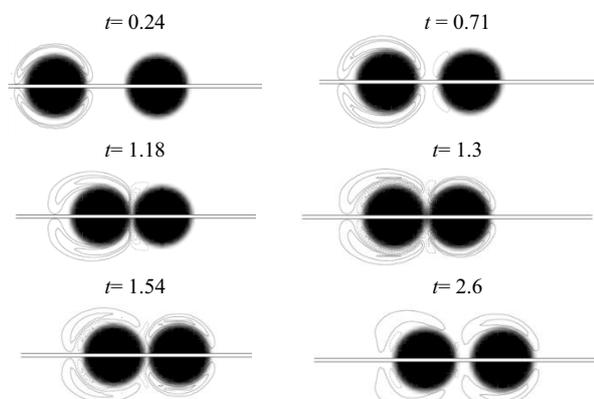
**Fig. 3.** Iso-vorticity contours from  $-4.25$  to  $4.25$  over time of two spheres bouncing with  $\rho_p/\rho = 8$ ,  $St = 140$  and  $Re \approx 175$ . Positive (resp. negative) values are continuous (resp. dashed) lines. Images are mirrored. The particle on the left (right) is labelled particle 1 (2).
