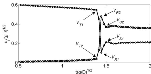
**Fig. 4.** Time evolution of the particle velocities (same case as in Fig. 3) during the bouncing of two spheres. The terminal velocity  $V_{Ti}$  and rebound velocities  $V_{Ri}$  and  $V_{Si}$  of particle  $i$  are represented.
