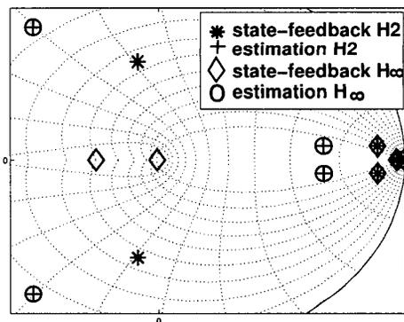
FIGURE 4: Closed-loop eigenvalue map for  $H_\infty$  and  $H_2$  syntheses.
