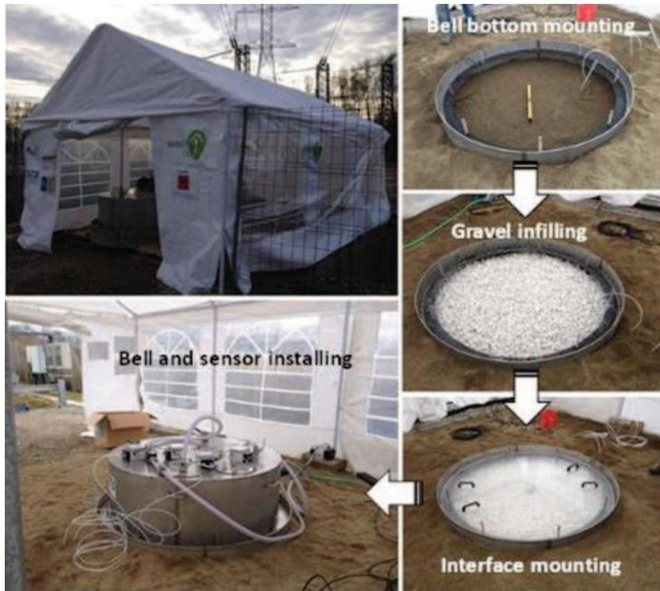
Figure 1 - View of the experimental set-up in the PISCO<sub>2</sub> facilities at Ponferrada. The sequence of pictures on right represents the installation of components.
