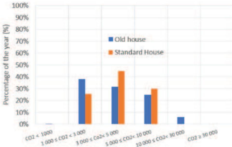
Figure 12- CO<sub>2</sub> concentration distribution in the building for the year, for an injection flux of 0.01 kg/s, a vadose permeability of  $5.10^{-11}$  m<sup>2</sup>, a slab permeability of  $2.10^{-13}$  m<sup>2</sup>
