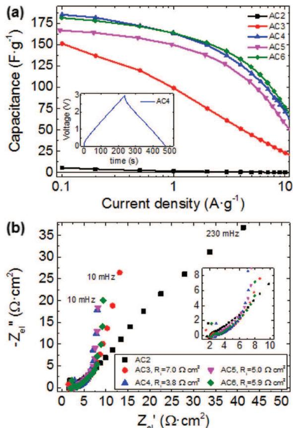
**Fig. 3.** (a) Capacitance of ACs in neat EMI-TFSI as a function of current density (inset - galvanostatic charge-discharge profile at  $1\text{ A}\cdot\text{g}^{-1}$ ); (b) Nyquist plot  $\text{Ohm}\cdot\text{cm}^2$  per electrode (inset - high frequency range).
