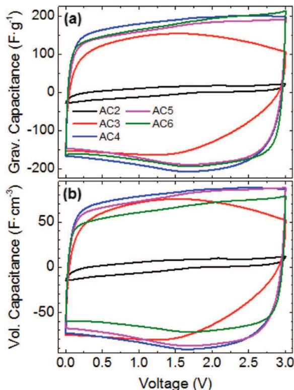
**Fig. 2.** Cyclic voltammograms of ACs from olive pits at a scan rate of  $5\text{ mV}\cdot\text{s}^{-1}$  in neat EMI-TFSI at room temperature [ $20^\circ\text{C}$ ] (a) gravimetric and (b) volumetric capacitance.
