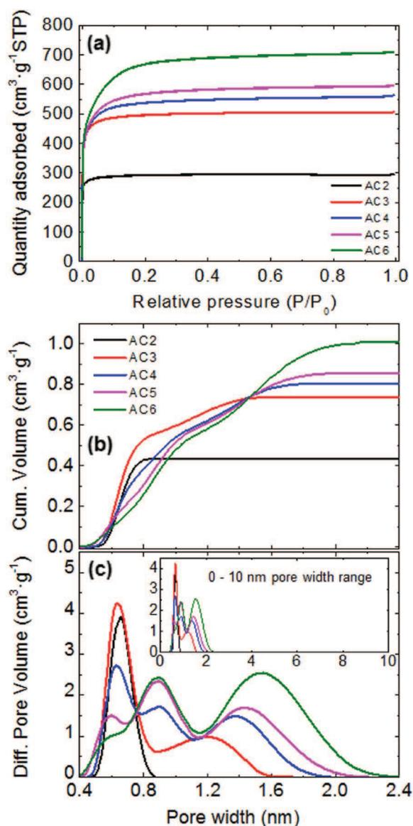
Fig. 1. (a) N<sub>2</sub> adsorption/desorption isotherms (b) cumulative (c) differential pore volume (dV/dlgL) vs pore size calculated by the 2D-NLDFT model.
