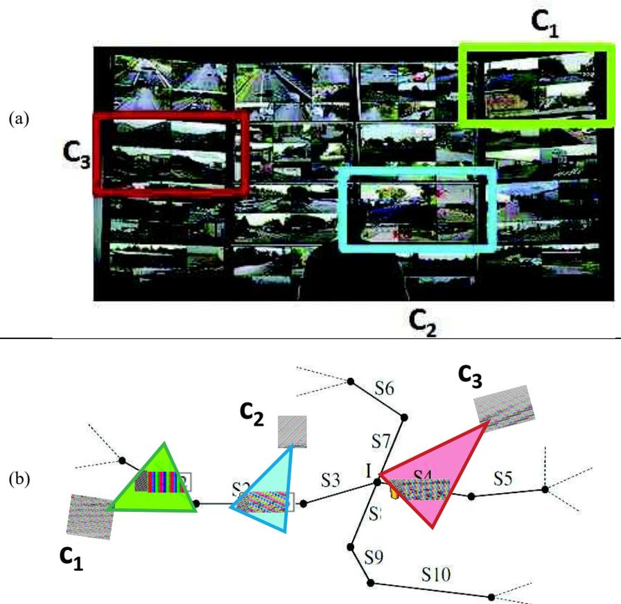
Figure 1. The lack of spatial organization on a video wall. (a) The video wall seen by operators. (b) The real positions of cameras on the road segments
