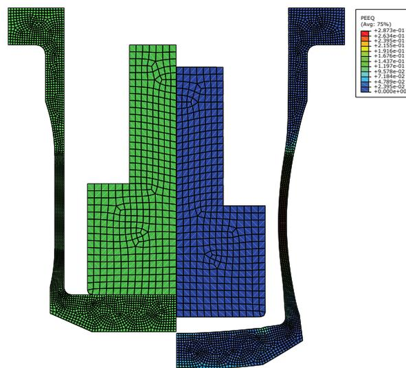
Figure 2: Two-dimensional axisymmetric tensile Finite Element Model: left is undeformed model, right is plastic strain after impact.
