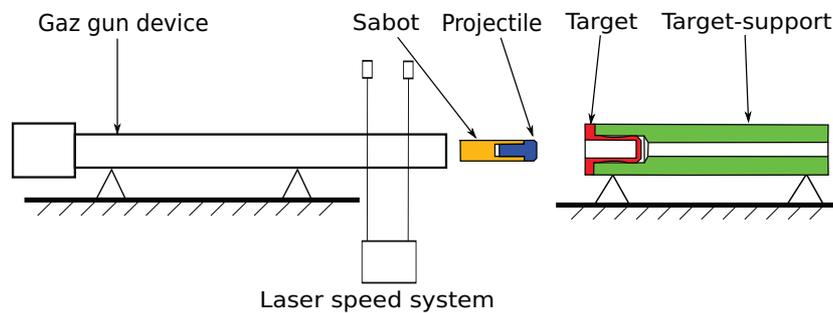
Figure 1: Layout of Taylor tensile facility using a gaz gun
