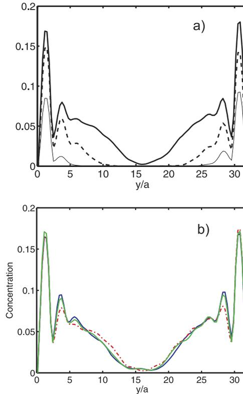
FIG. 9. Solid volume fraction profiles of a laminar channel flow after the particle migration towards the wall is completed. (a)  $Re = 1400$  and  $\phi_b = 1$  (thin line),  $2.5$  (dashed), and  $5\%$  (solid thick line). (b)  $\phi_b = 5\%$  and  $Re = 1400$  (dashed-dotted),  $1200$  (light gray — green online), and  $1000$  (dark gray — blue online).
