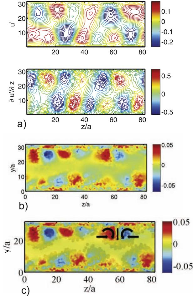
FIG. 13. (a) Contours of the streamwise velocity fluctuations scaled by  $\langle U \rangle$  followed by the spanwise velocity gradient scaled by the average flow shear rate. (b) Contours of streamwise vorticity scaled by the average shear rate. All these contours correspond to averages in the streamwise direction at the same time  $t = 200H/\langle U \rangle$  at  $Re = 1400$ . In (c), the secondary flows are superposed with the particle front view of panel (a).
