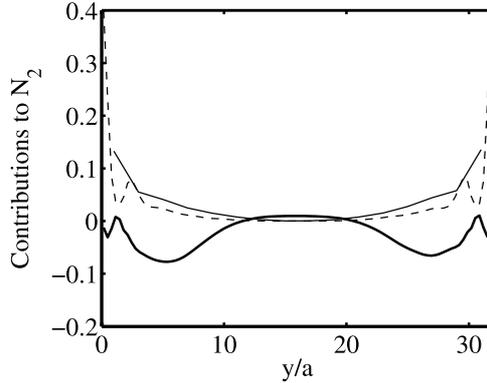
FIG. 12. Profiles of the contributions to the second normal stress difference scaled by the wall shear stress at  $Re = 1400$  and  $t = 70H/\langle U \rangle$ . Thick solid line:  $v'^2 - w'^2$ . Thin solid line:  $S_{22}^{sl} - S_{33}^{sl}$ . Dashed line: prediction of  $S_{22}^{sl} - S_{33}^{sl}$  from the single particle in unbounded pure shear flow considering local  $Re_p$  and shear rate.
