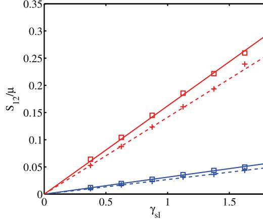
FIG. 6. Stresslet-shear rate diagram in Poiseuille flow. Square and plus symbols are, respectively, for  $Re = 500$  and  $10^{-3}$ . Dark and light gray (online blue and red) colors are for  $\phi_b = 1\%$  and  $5\%$ , respectively. The lines are obtained from linear fitting for each case.
