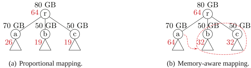
Figure 2: Mapping strategies. Sequential peaks of active memory are in black. The number of processors associated with each subtree is in red. In (b), the arrow is a scheduling constraint.
