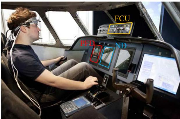
Figure 1: ISAE 3-axis motion flight simulator. FCU: Flight Control Unit. PFD: Primary Flight Display. ND: Navigation Display.
