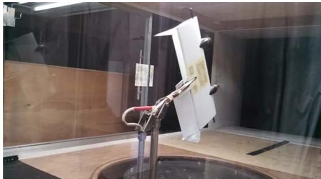
Fig. 1. *MAVion* under wind tunnel testing.
