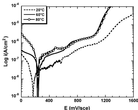
Fig. 4. Potentiodynamic curves obtained on graphite in  $H_3PO_4$  at 20, 60 and  $80^\circ C$ .
