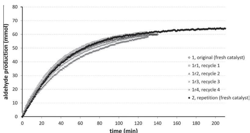
**Fig. 2.** Aldehyde production\* during the consecutive cycles with the reference TPP@CCM in standard conditions. \*Calculated from syngas consumption after gas induction (excluding the first 20 s corresponding to gas absorption).
