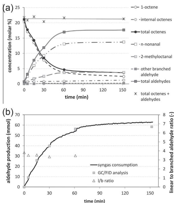
**Fig. 3.** Evolution of reactants and products during the reaction performed at 1600 rpm (other parameters set as per standard conditions): (a) evolution of the concentrations in the organic phase and overall mass balance, (b) comparison of the produced aldehydes from GC/FID analysis\*\* and from syngas consumption after gas induction and time evolution of the l/b ratio. \*\*Assuming a uniform composition of the organic phase (in the bulk and within the objects).
