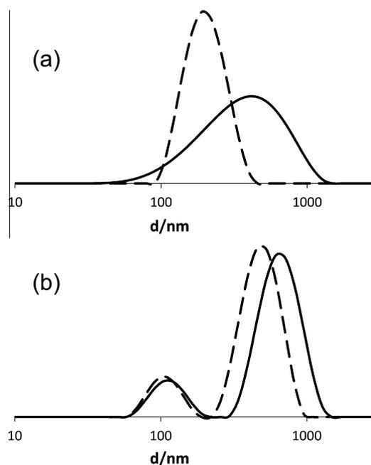
Fig. 5. DLS analysis of the recovered organic phase after stirring the TPP@CCM with *n*-decane for 2.5 h at 90 °C (measurements carried out at room temperature): (a) without Rh and (b) with Rh (P/Rh = 4). In both cases, the solid curve was recorded immediately after recovery; the dashed curve was recorded after one week standing at room temperature.
