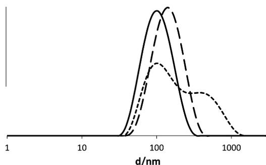
Fig. 4. DLS analysis of the recovered organic phase after the catalytic runs 2, 7a and 7b in Table 2. Stirring speed (rpm): 1200 (solid), 1400 (dashed), and 1600 (dotted).
