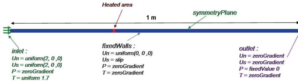
**Fig. 1** Geometry and boundary conditions of the domain.
