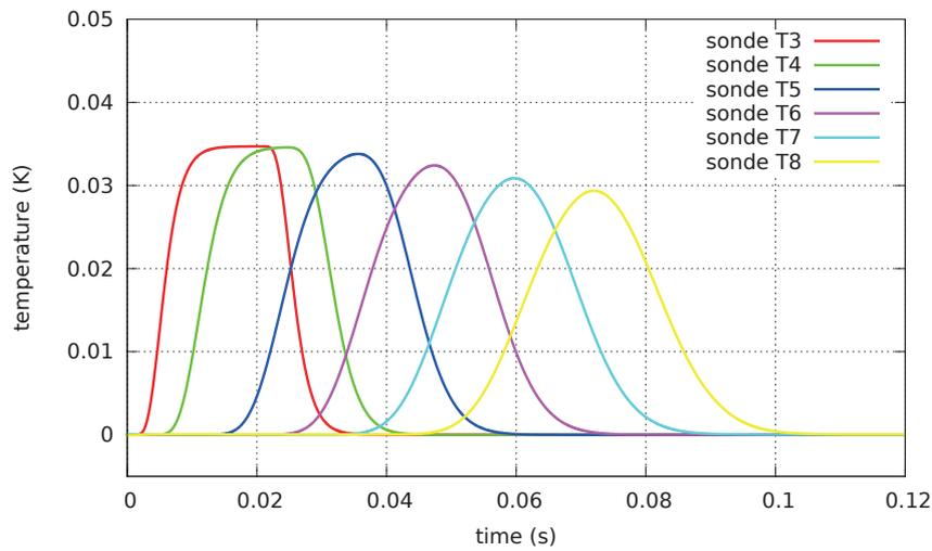
**Fig. 5** Transient temperature profile recorded by several probes placed along the tube in case of a forced convection flow at 8 m/s.
