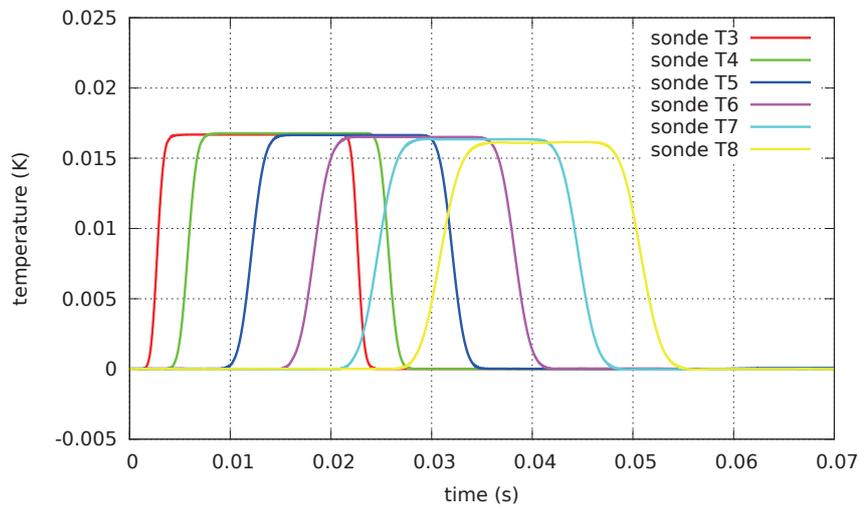
**Fig. 6** Transient temperature profile recorded by several probes placed along the tube in case of a forced convection flow at 16 m/s.
