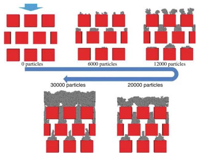
**Fig. 10** Simulation of the capture of particles in staggered pillars geometry
