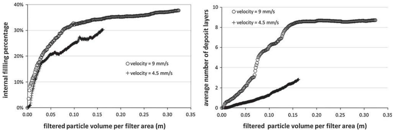
**Fig. 7** Variation of the internal filling and of the number of deposit layers as a function of the volume of filtered particles per filter area (the product of the filtration time, the fluid velocity and the volume fraction of the dispersion) for a fluid velocity of 4.5 and  $9 \text{ mm s}^{-1}$
