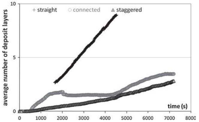
**Fig. 5** Variation with time of the internal filling percentage (ratio of the surface occupied by particles over the total available surface within the porous media) and of the average number of deposit layers (ratio of the mean deposit thickness in the upstream zone over the
