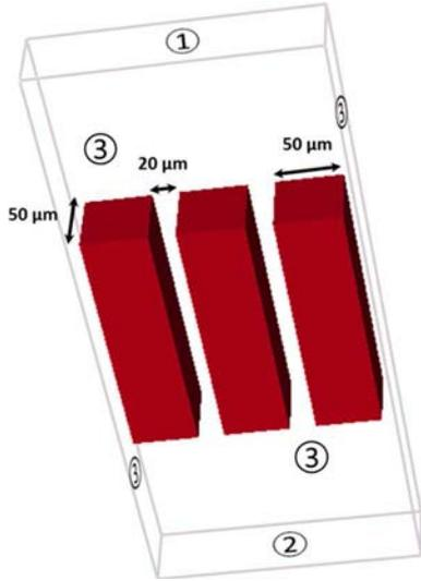
**Fig. 3** Scheme of the model for numerical simulation (surface 1 inlet, surface 2 outlet, surfaces 3 periodic conditions)
