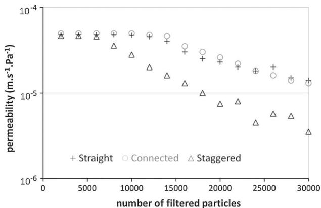
**Fig. 12** Evolution of the permeability as a function of the number of particles filtered through the geometries with straight channel, connected channels or staggered pillars (30,000 filtered particles correspond to 40 s of filtration during experiments)
