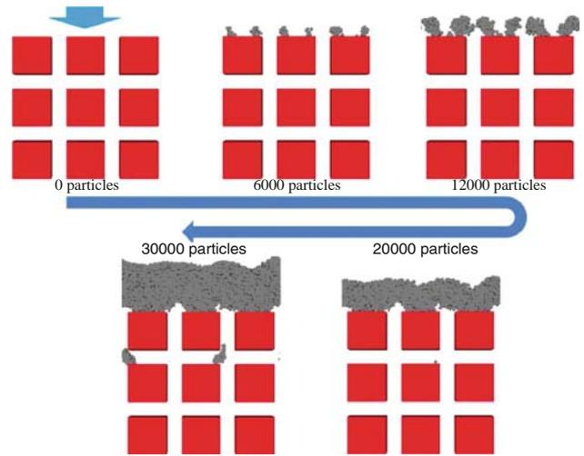
**Fig. 9** Simulation of the capture of particles in connected channel geometry
