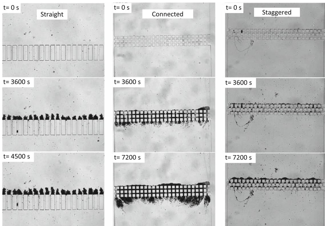
**Fig. 4** Effect of microchannels geometry on the plugging. Images are taken at different times during the filtration (filtration velocity from the top to the bottom) of 5  $\mu\text{m}$  latex particles with a volume fraction
