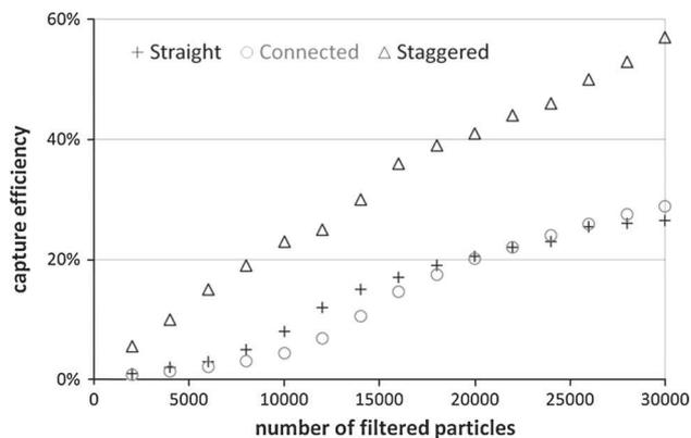
**Fig. 11** Evolution of the capture efficiency as a function of the number of particles filtered through the geometries with straight channel, connected channels or staggered pillars (30,000 filtered particles correspond to 40 s of filtration during experiments)
