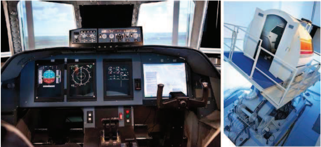
Figure 1: Photos of the ISAE flight simulator. Cockpit view (left panel) and view from outside the simulator (right panel). Participants flew the aircraft from the left seat.
