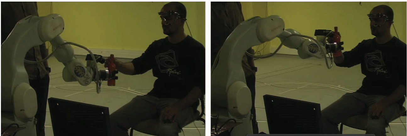
Fig. 3. The robot's and human's posture while passing the bottle in the Motion-1 (left) and Motion-2 (right)
