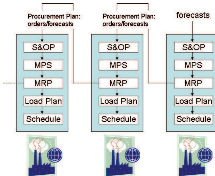
Figure 1. Point-to-point coordination in a SC using MRPII
