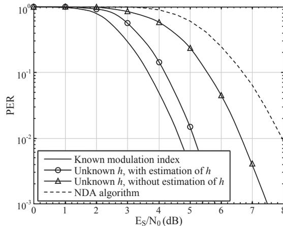
Figure 6. Proposed receiver compared with the algorithm presented in Section 3 when the modulation index is known and the nondata-aided (NDA) algorithm in packet error rate.
