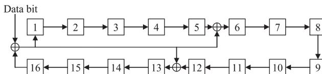
Figure 2. Example of iterative cyclic redundancy check computation with the generator polynomial  $G(x) = x^{16} + x^{12} + x^5 + 1$ .  $\oplus$  represent XOR and are placed according to the generator polynomial. The numbered boxes contain the derived cyclic redundancy check bits.
