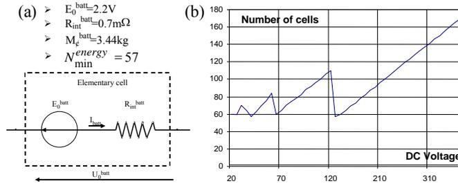
**Fig. 6.** Characteristics of the battery cells
