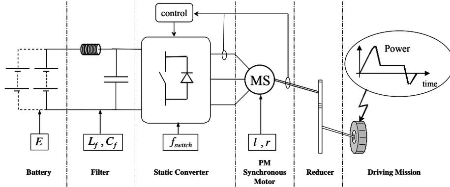
**Fig. 4.** Synoptic of the electric vehicle model
