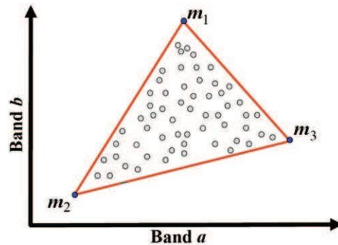
**Fig. 1.** Geometrical formulation of spectral mixture analysis (SMA). The scatterplot represents the data observed in a 2-D space. The mixed pixels (gray circles) belong to the simplex (simplest geometric figure that is not degenerate in  $n$ -dimensions), whose vertices are the 3 endmembers. SMA algorithms exploit different properties of the simplex.
