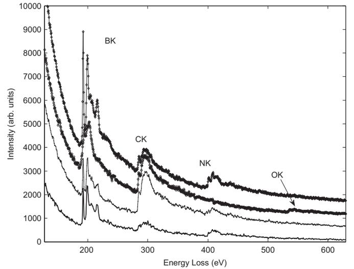
**Fig. 3.** Typical EELS spectra extracted from the  $64 \times 64$  spectrum image in Fig. 2. Boron, carbon, nitrogen and oxygen K edges are represented.
