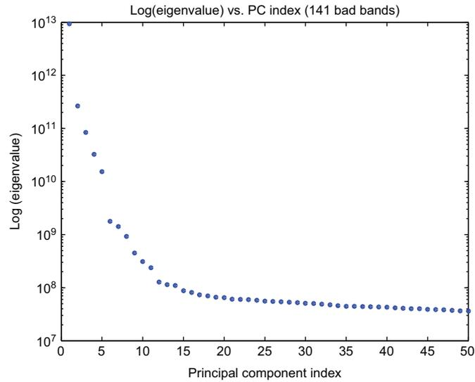
**Fig. 4.** Principal component eigenvalues for the analyzed spectrum-image arranged in a decreasing order (depicted in logarithmic scale). The threshold between eigenvalues associated signal and those associated with noise is not easy to determine. Indeed, there is no drastic drop in the eigenvalue distribution. In this work, the intrinsic dimensionality of the data is estimated around 7.
