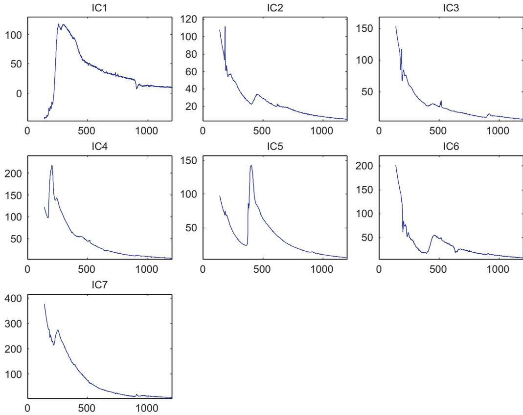
**Fig. 6.** Spectral components extracted by CubICA. Some components are completely different from the reference spectra and have no physical meaning. The corresponding maps are depicted in Fig. 7.
