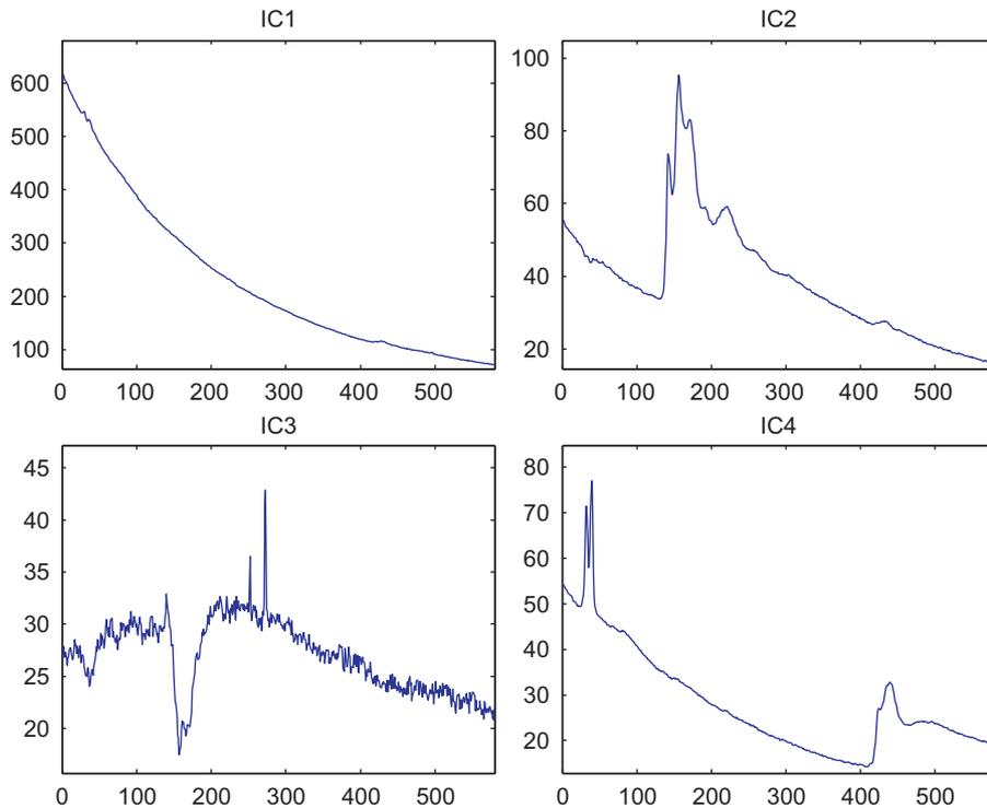
**Fig. 8.** Spectral components extracted by CubICA with a restricted 430–800 eV energy range. In this case the unmixing is quite satisfactory but only 4 physical EELS spectra are identified. The corresponding maps are depicted in Fig. 9.
