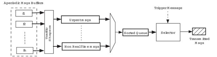
Fig. 3. Arbitration mechanism of aperiodic traffic in the slave
