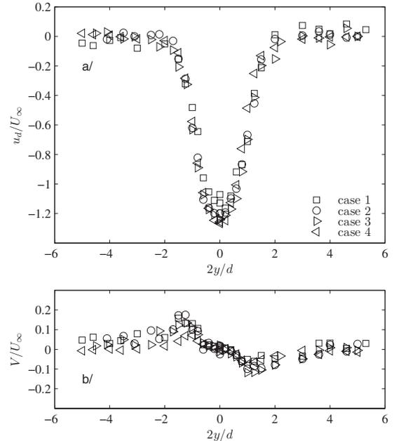
FIG. 5. Transverse profiles of the streamwise  $U$  (a) and transverse  $V$  (b) mean velocities in the near wake at  $2x/d=2$ . ( $\square$ ) Case 1 ( $Re_S=110$ ,  $I_t=0.45$ ,  $Re_\lambda=35$ ). ( $\circ$ ) Case 2 ( $Re_S=220$ ,  $I_t=0.38$ ,  $Re_\lambda=53$ ). ( $\triangleright$ ) Case 3 ( $Re_S=670$ ,  $I_t=0.26$ ,  $Re_\lambda=76$ ). ( $\triangleleft$ ) Case 4 ( $Re_S=1080$ ,  $I_t=0.26$ ,  $Re_\lambda=85$ ).
