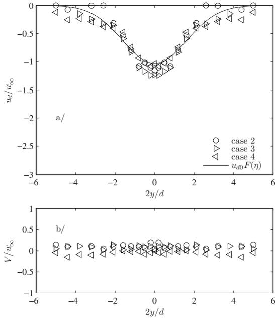
FIG. 6. Transverse profiles of the streamwise  $U$  (a) and transverse  $V$  (b) mean velocities at  $2x/d=6$ . ( $\circ$ ) Case 2 ( $Re_S=220$ ,  $I_t=0.38$ ,  $Re_\lambda=53$ ). ( $\triangleright$ ) Case 3 ( $Re_S=670$ ,  $I_t=0.26$ ,  $Re_\lambda=76$ ). ( $\triangleleft$ ) Case 4 ( $Re_S=1080$ ,  $I_t=0.26$ ,  $Re_\lambda=85$ ). Continuous line:  $u_d(x,y)=u_{d0}(x)\exp(-\eta^2/2)$  for case 4.
