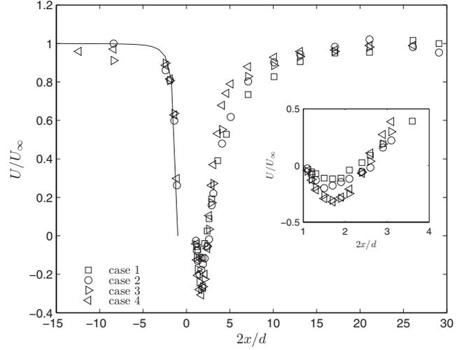
FIG. 4. Mean streamwise velocity along the vertical axis of the sphere. ( $\square$ ) Case 1 ( $Re_S=110$ ,  $I_t=0.45$ ,  $Re_\lambda=35$ ). ( $\circ$ ) Case 2 ( $Re_S=220$ ,  $I_t=0.38$ ,  $Re_\lambda=53$ ). ( $\triangleright$ ) Case 3 ( $Re_S=670$ ,  $I_t=0.26$ ,  $Re_\lambda=76$ ). ( $\triangleleft$ ) Case 4 ( $Re_S=1080$ ,  $I_t=0.26$ ,  $Re_\lambda=85$ ). Continuous line: prediction for potential flow around a sphere.
