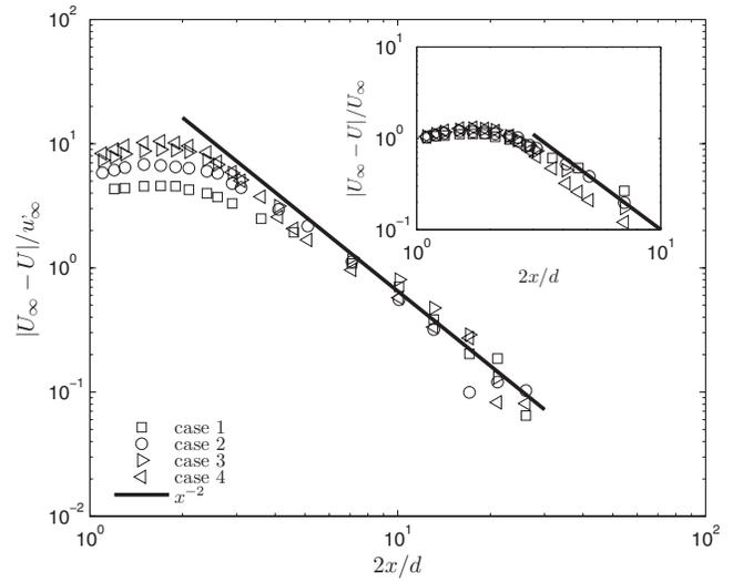
FIG. 7. Axial evolution of the mean velocity defect normalized by  $u'_\infty$  or  $U_\infty$ . ( $\square$ ) Case 1 ( $Re_S=110$ ,  $I_t=0.45$ ,  $Re_\lambda=35$ ). ( $\circ$ ) Case 2 ( $Re_S=220$ ,  $I_t=0.38$ ,  $Re_\lambda=53$ ). ( $\triangleright$ ) Case 3 ( $Re_S=670$ ,  $I_t=0.26$ ,  $Re_\lambda=76$ ). ( $\triangleleft$ ) Case 4 ( $Re_S=1080$ ,  $I_t=0.26$ ,  $Re_\lambda=85$ ).
