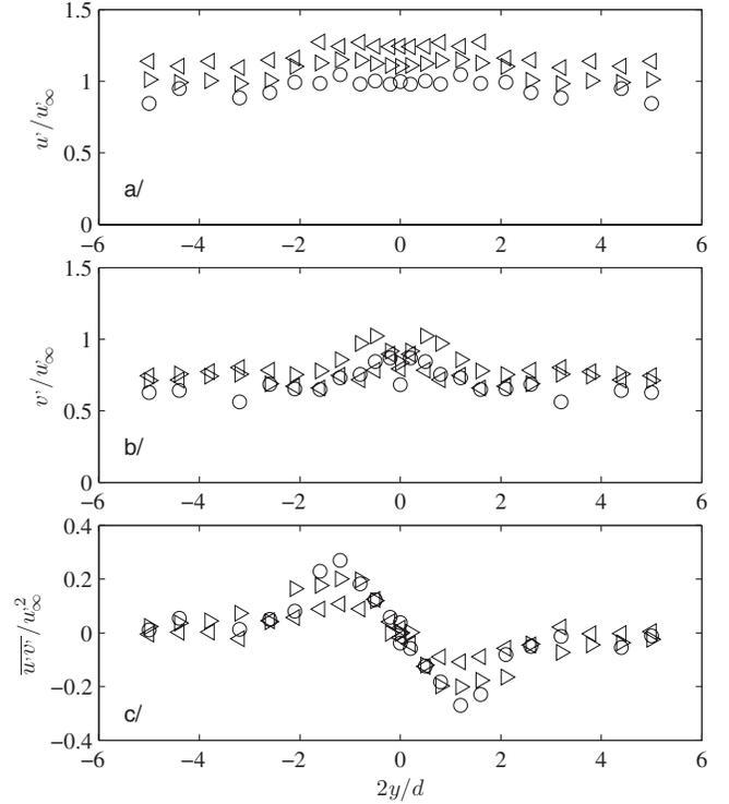
FIG. 11. Transverse profiles of the fluctuations normalized by the incident turbulent velocity  $u'_\infty$  at  $2x/d=6$ . (a) Standard deviation of the longitudinal velocity  $u'$ , (b) standard deviation of the transversal velocity  $v'$ , and (c) shear stress  $\overline{u'v'}$ . (○) Case 2 ( $Re_S=220$ ,  $I_t=0.38$ ,  $Re_\lambda=53$ ). (△) Case 3 ( $Re_S=670$ ,  $I_t=0.26$ ,  $Re_\lambda=76$ ). (▽) Case 4 ( $Re_S=1080$ ,  $I_t=0.26$ ,  $Re_\lambda=85$ ).
