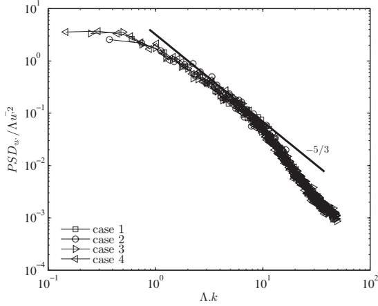
FIG. 3. Spectra of the longitudinal velocity of the incident turbulence. ( $\square$ ) Case 1 ( $Re_S=110$ ,  $I_t=0.45$ ,  $Re_\lambda=35$ ). ( $\circ$ ) Case 2 ( $Re_S=220$ ,  $I_t=0.38$ ,  $Re_\lambda=53$ ). ( $\triangleright$ ) Case 3 ( $Re_S=670$ ,  $I_t=0.26$ ,  $Re_\lambda=76$ ). ( $\triangleleft$ ) Case 4 ( $Re_S=1080$ ,  $I_t=0.26$ ,  $Re_\lambda=85$ ).
