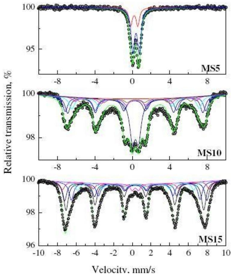
Figure 1 Mössbauer spectra of CoFe<sub>2</sub>O<sub>4</sub> at 295 K for different milling time.
