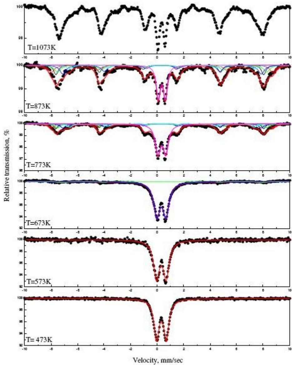
Figure 3 RT Mössbauer spectra of all synthesised  $\text{Co}_2\text{FeO}_4$  samples.
