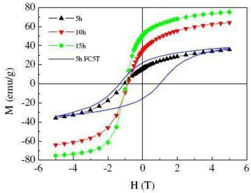
Figure 2 ZFC–isothermal magnetization(5 K) of the milled  $\text{CoFe}_2\text{O}_4$  and FC (5 T) for the 5 h milled sample.
