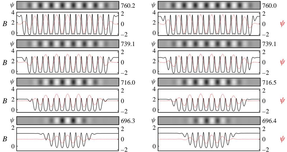
FIGURE 2. (Colour online) Solution profiles along the stable upper convecton branches  $L^+$  (left column) and  $L^-$  (right column) in figure 1 at the Rayleigh numbers indicated on the right in terms of contours of the streamfunction  $\psi$  (upper panels) and the profiles of  $\psi(x, 1/2)$  (red, dashed) and the resulting vertical magnetic field  $B \equiv 1 + A_x(x, 1/2)$  (black, solid).
