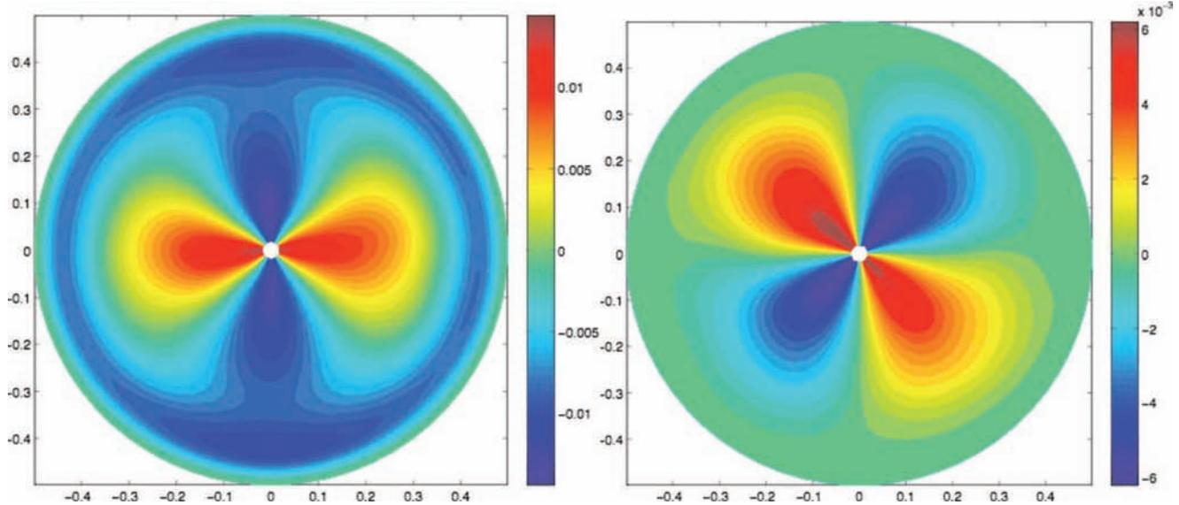
FIG. 4. (Color online) Map of the secondary anisotropy  $\langle v_r^2 \rangle - \langle v_\theta^2 \rangle$  (left) and cross correlation  $\langle v_r v_\theta \rangle$  (right), both normalized by  $V_i^2$ .
