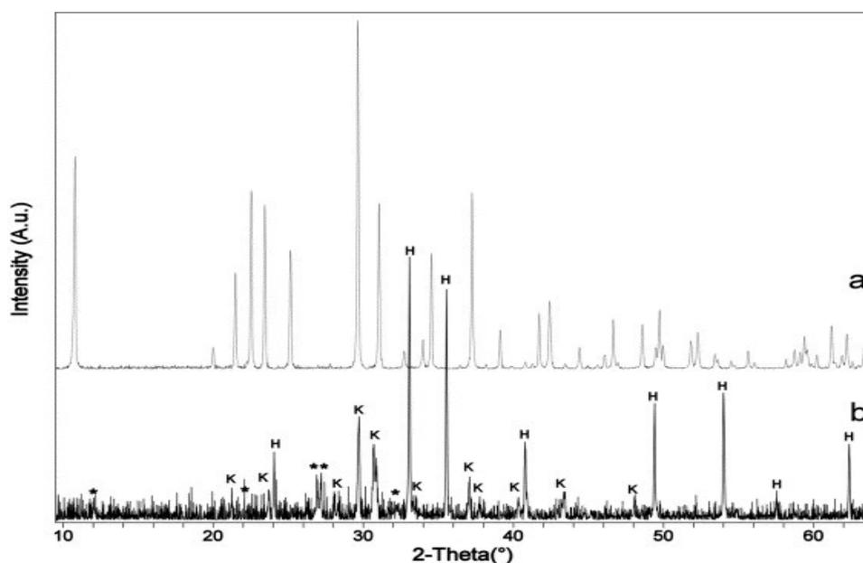
The X-ray diffraction pattern (Fig. 1) for yavapaiite heated to 1000°C in air shows the presence of two main phases, hematite  $\text{Fe}_2\text{O}_3$  (ICDD-PDF 60-8558) and arcanite  $\text{K}_2\text{SO}_4$  (ICDD-PDF 64-3139). However, some unidentified peaks are also observed, indicating the presence of other decomposition products.
